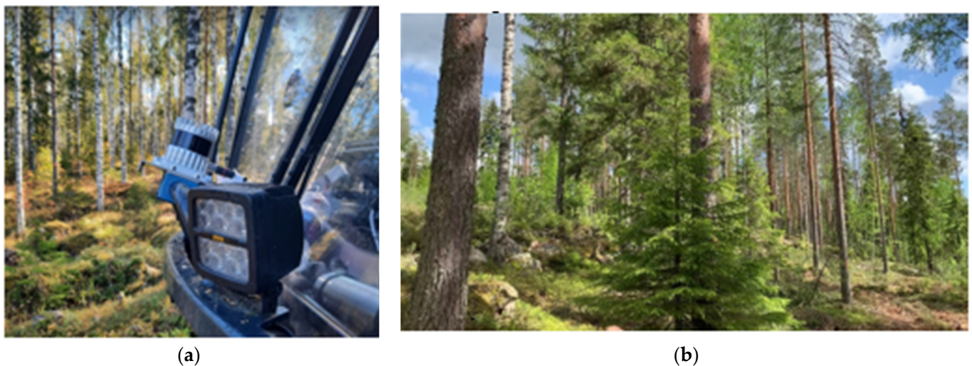
Figure 3. The Ouster LiDAR OS0 on the Ponsse Scorpion (a) and the view from the test forest (b).
