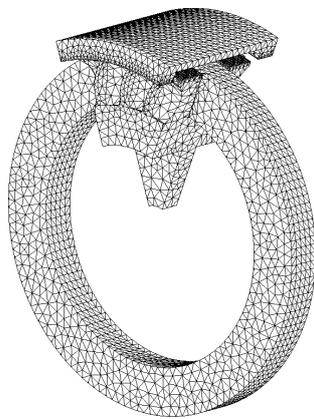
**Figure 3.** The partial finite element analysis model.
