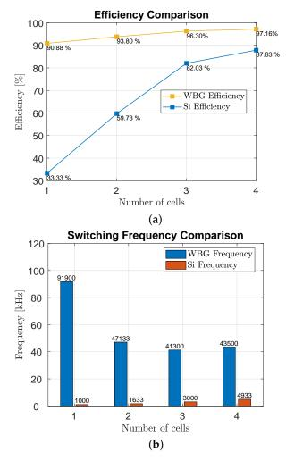
**Figure 12.** Comparison of WBG and Si devices for a 40kW load: (**a**) Efficiency comparison. (**b**) Frequency comparison.
