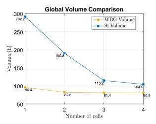
Figure 11. Volume comparison of WBG and standard devices for a 40-kW load.
