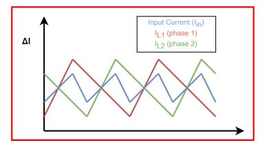
Figure 3. Current ripples waveforms of a two-phase interleaved boost converter.
