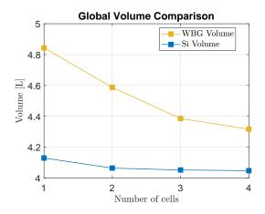
Figure 9. Volume comparison of WBG and standard devices for a 2-kW load.
