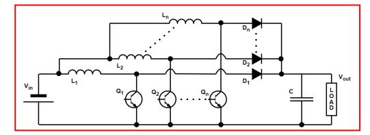
Figure 2. Interleaving of a n-cell Boost converter.
