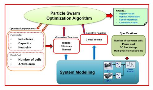
Figure 7. A global optimization methodology under multiphysical constraints.
