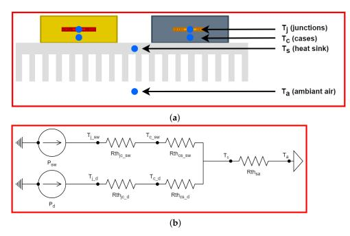
**Figure 8.** Thermal modeling of two semiconductors sharing the same heat sink: (**a**) Thermal dissipation setup scheme. (**b**) Equivalent thermal circuit of the adopted thermal management.
