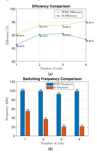
**Figure 10.** Comparison of WBG and Si devices for a 2kW load: (a) Efficiency comparison. (b) Frequency comparison.
