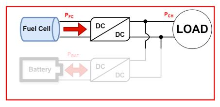
Figure 4. Parallel hybrid power source architecture.
