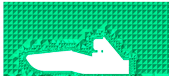
Figure 12. Mesh distribution of densified area.
