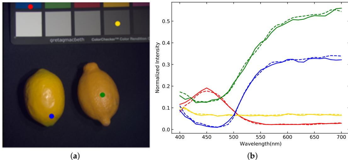
**Figure 8.** (a) RGB image of Fake and Real Lemons in CAVE with four selected points. (b) The spectral curves of four points obtained by our method and the ground truth are plotted by the dashed lines and solid lines, respectively.
