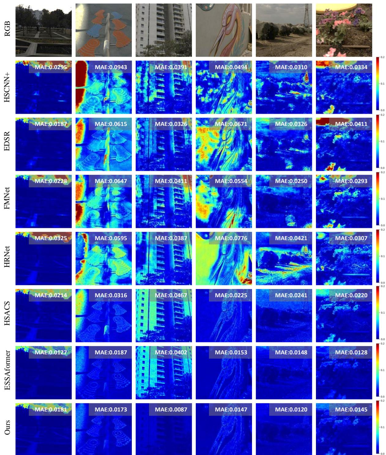
**Figure 9.** Qualitative results of six example images from the validation data in NTIRE2022. The initial row displays the RGB images, while the subsequent rows (second to eighth) depict the absolute error maps corresponding to different SSR methods. The MAE value on the top right corner of each absolute error map represents the mean absolute error of that map.
