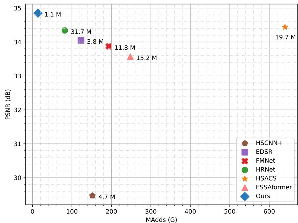
**Figure 1.** Comparison of our proposed TCSSA model with other SSR models using the CAVE dataset. The horizontal axis represents multiply-add operations (MAdds), while the vertical axis depicts peak signal-to-noise ratio (PSNR). The points in the figure are labeled as the number of parameters. Our TCSSA approach exhibits a better tradeoff between its computational complexity (numbers of parameters and MAdds) and PSNR.
