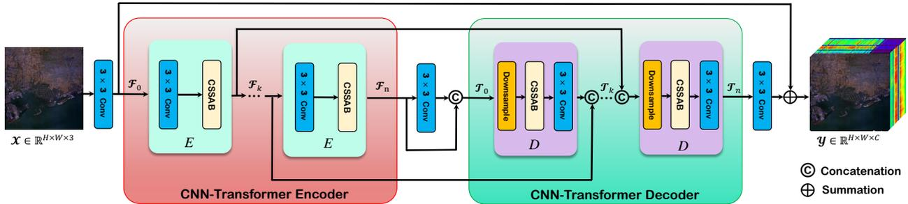
**Figure 2.** The structure of the proposed TCSSA, primarily comprising a CNN-Transformer encoder and a CNN-Transformer decoder.
