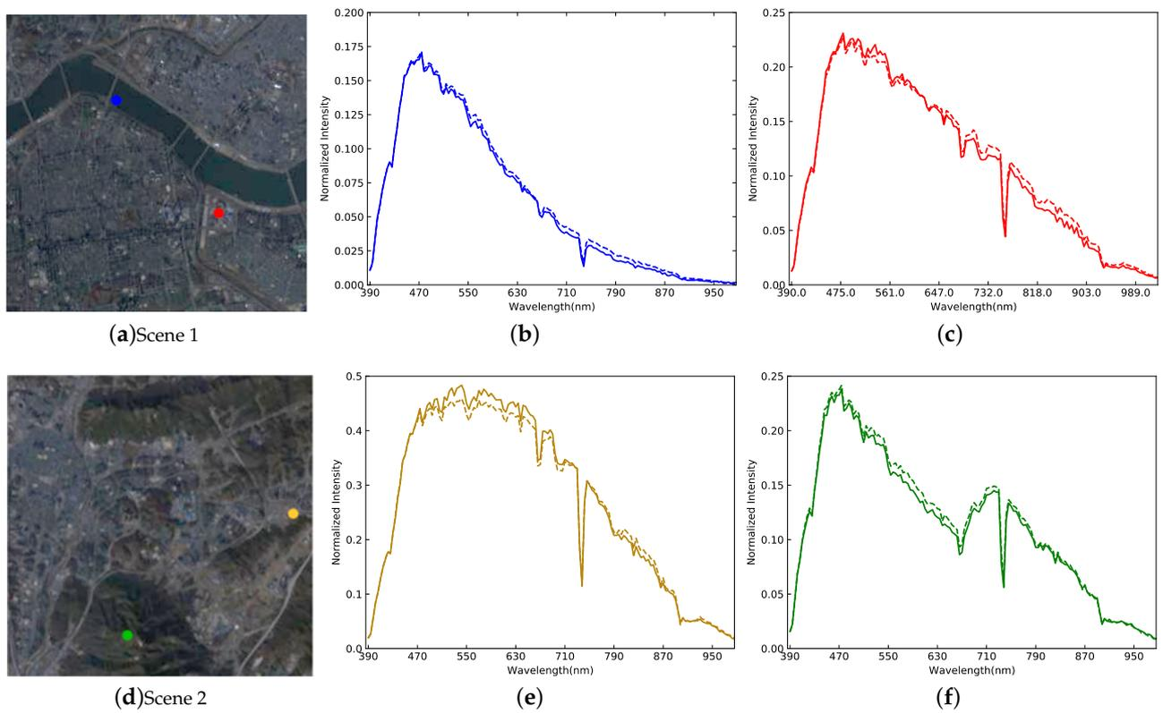
**Figure 6.** (a,d) are two scenes from the validation data in GF5, while (b,c) are the spectral curves of the blue and red points in (a) and (e,f) are the spectral curves of the yellow and green points in (d). The solid and dashed lines represent the ground truth and the spectral signature recovered by the proposed method.
