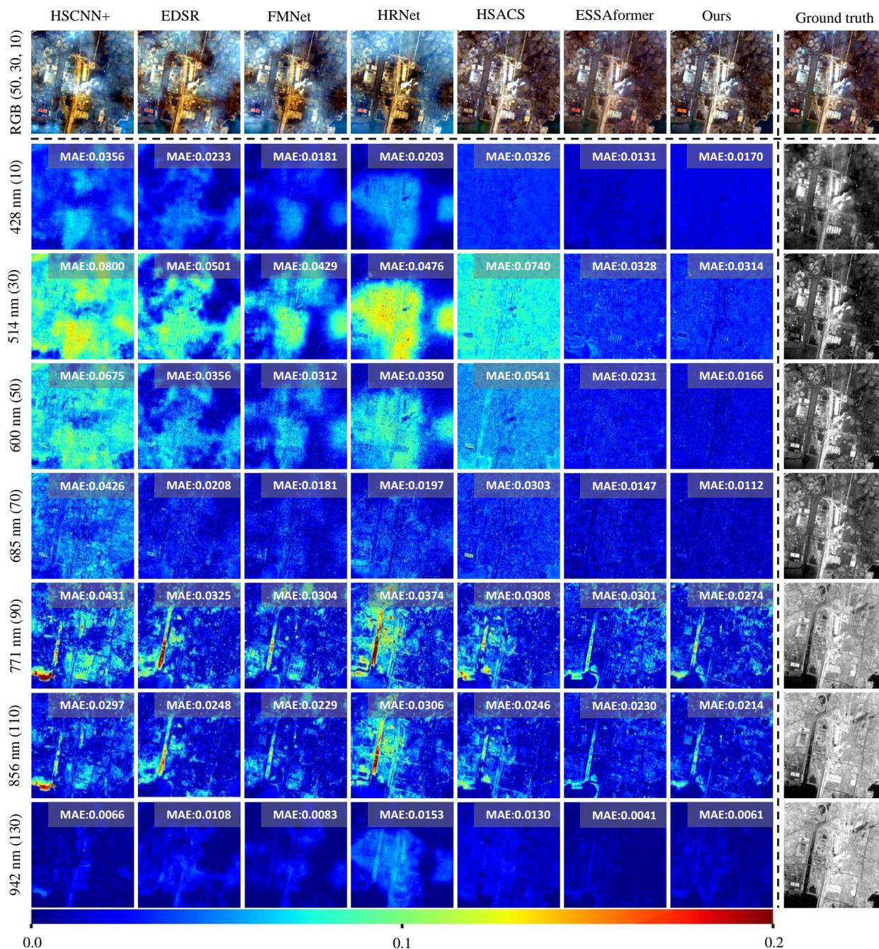
**Figure 5.** Qualitative results of an example image from the test data in GF5. The top row displays the restored true-color RGB composites of bands 50 (600 nm), 30 (514 nm), and 10 (428 nm) by all methods and ground truth. The second to eighth rows are the results of absolute error maps corresponding to seven reconstructed spectral bands at different wavelengths and ground truth. The MAE value on the top right corner of each absolute error map represents the mean absolute error of that map.
