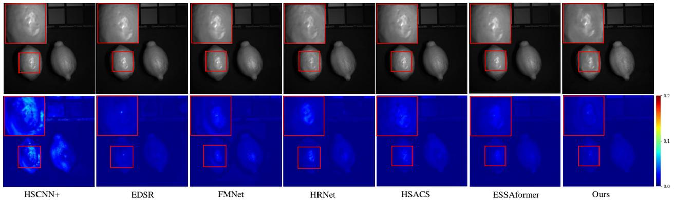
**Figure 7.** Qualitative results of lemons in CAVE. The **top** row exhibits reconstructed images at band 31 obtained from different SSR methods, while the **bottom** row displays the corresponding mean absolute error maps.
