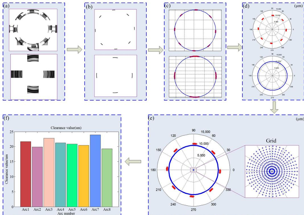
**Figure 14.** Flowchart of calculating the assembly fit clearance values: (a) Experimental image of parts; (b) Extract the target edges of the images; (c) Calculate centers using the least square fit; (d) Convert to polar coordinates; (e) Calculate the assembly alignment position based on uniformity assembly using grid search; (f) Calculate the mean fit clearance values.
