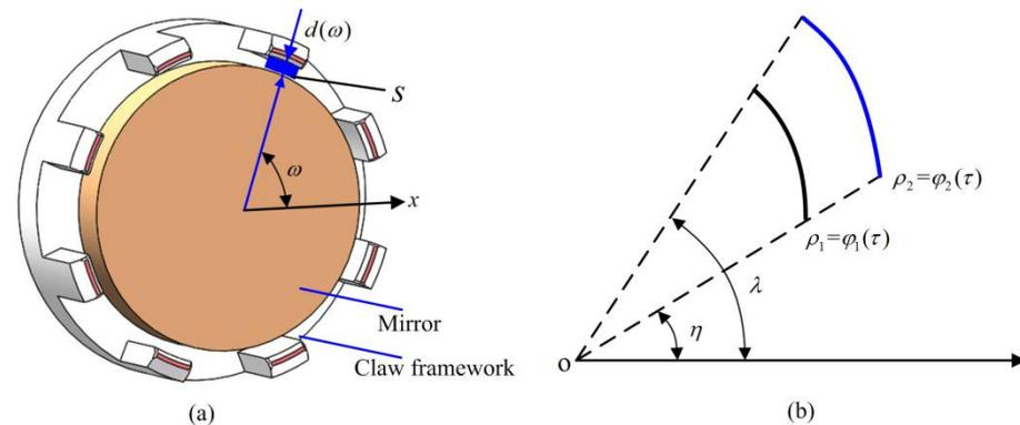
**Figure 13.** Fit clearance values: (a) Fit clearance value about claw framework and mirror; (b) Arcs in polar coordinates.
