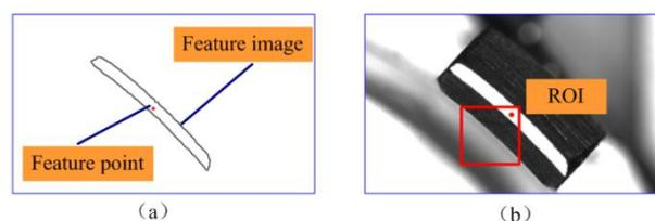
**Figure 7.** Feature point and ROI: (a) Feature image and feature point; (b) The ROI of the image of one arc structure.
