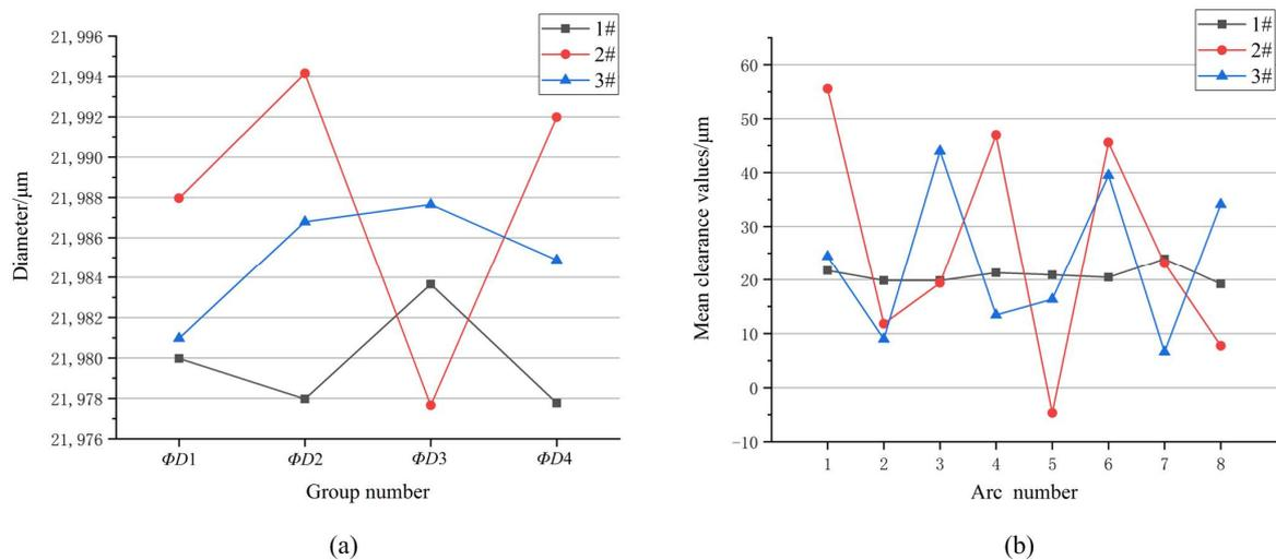
**Figure 15.** Grouping diameters and fit clearance values: (a) Diameter results for claw framework 1#, 2#, 3# (b) Predictive assembly means fit clearance values for 1#, 2#, 3#.
