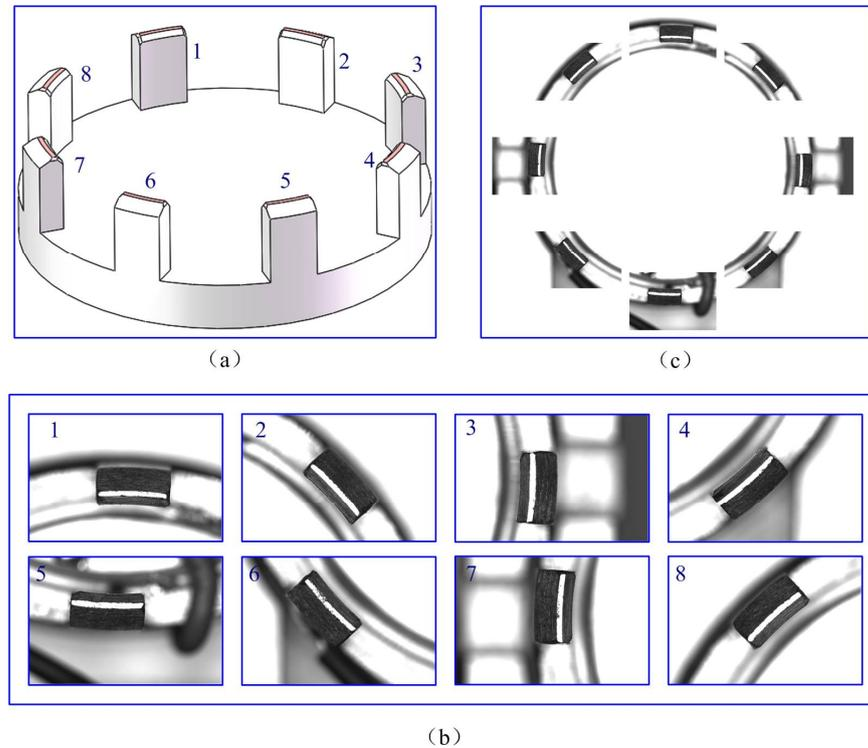
**Figure 4.** Experimental image of a claw framework: (a) Structure number; (b) Partial images; (c) The mosaic image.
