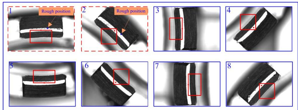
Figure 11. ROI extraction image of a part.
