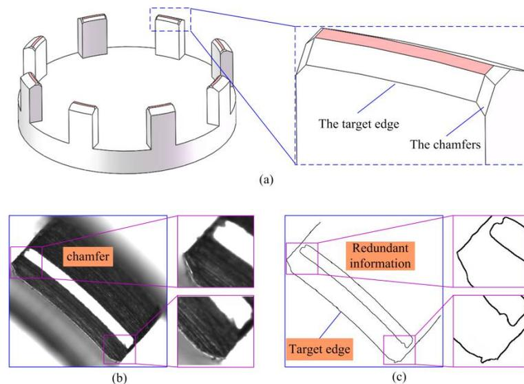
**Figure 6.** The target edge with the redundant chamfers information: (a) The chamfers of arc structure; (b) The chamfers image; (c) Redundant information between the target edge.
