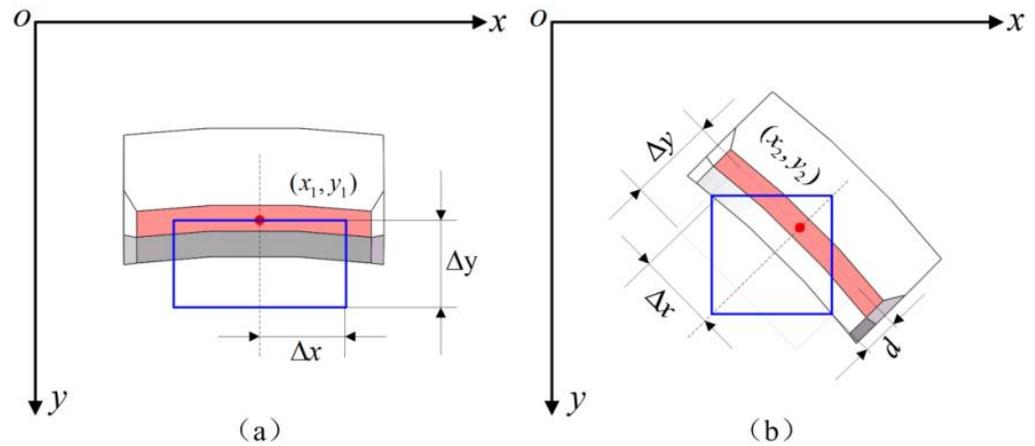
**Figure 10.** The relationship between feature point and ROI: (a) The ROI of the vertical direction arc structure; (b) The ROI of the oblique direction arc structure.
