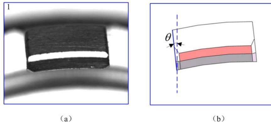
**Figure 9.** Deflection angle relative to the ideal position: (a) Image of the No.1 arc structure; (b) The rotation angle of the structure.
