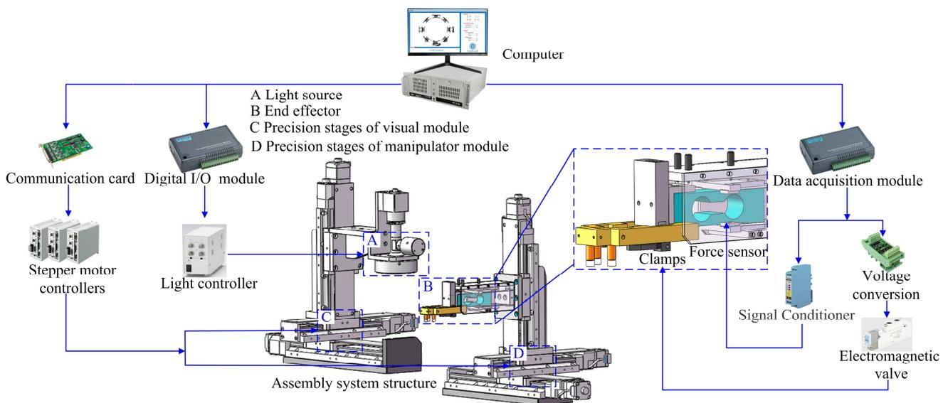
Figure 3. Hardware relationships of assemble system.
