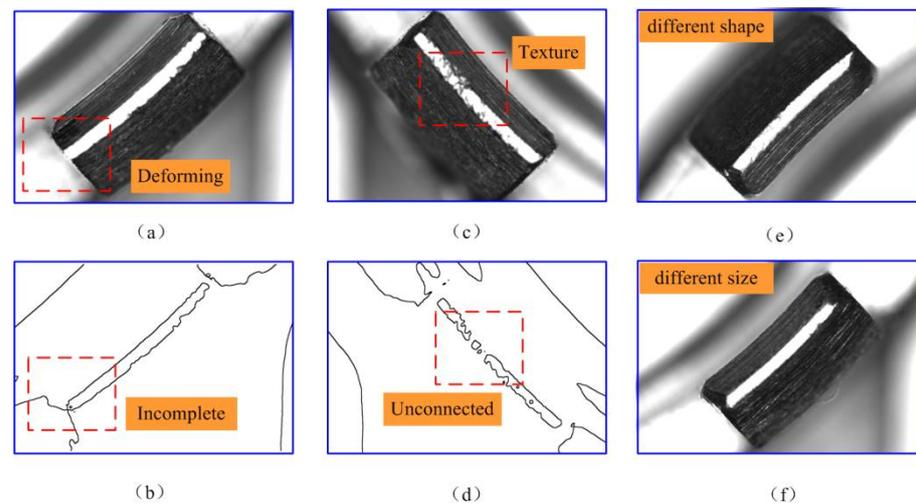
**Figure 8.** Structural deformation and processing texture of the feature image: (a) The deforming part; (b) The image preprocess result of the deforming part; (c) The part with machining texture; (d) The image preprocess result of the part with machining texture. (e) The feature image has a different shape. (f) The feature image has a different size.
