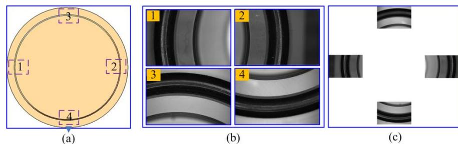
**Figure 5.** Experimental image of a mirror: (a) Image acquisition position; (b) Partial images; (c) the mosaic image.
