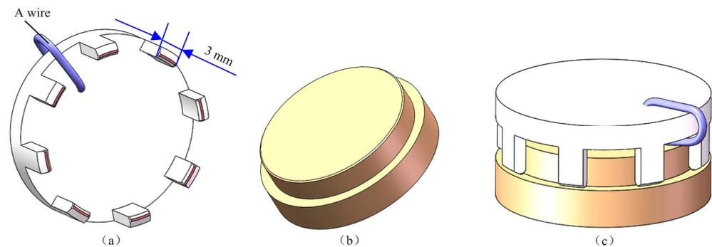
**Figure 1.** Parts and assembled component: (a) Claw framework; (b) Mirror; (c) Assembled component.
