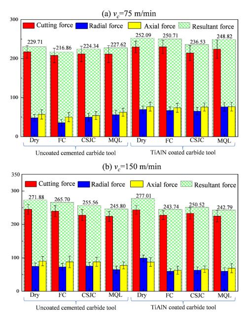
**Figure 5.** Measured cutting force, radial force, and axial force during the turning process of Ti-6Al-4V under dry and various cooling conditions at different cutting speeds: (**a**) 75 m/min and (**b**) 150 m/min.
