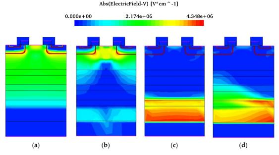
**Figure 12.** Electric field distribution transfer for SEB with buffer layer design: (**a**) 1 ps; (**b**) 10 ps; (**c**) 1000 ps; (**d**)  $10^{-7}$  s.
