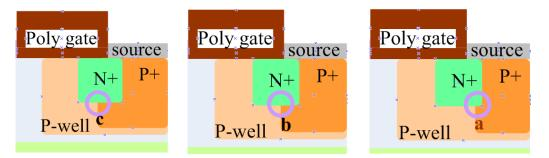
Figure 7. Schematic diagram of the expansion positions of different P+ body contact areas.
