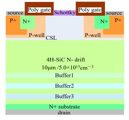
Figure 13. Device structure after comprehensive reinforcement optimization.
