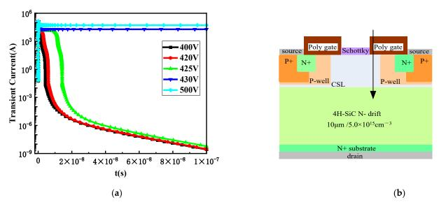
**Figure 5.** (a) Transient current curves of heavy ions incident from position B at different biases; (b) incident position B.
