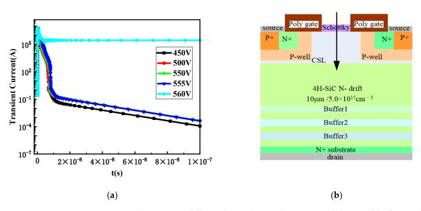
**Figure 10.** (a) Curves at different bias voltages after optimized design of buffer2 and buffer3; (b) incident position A.
