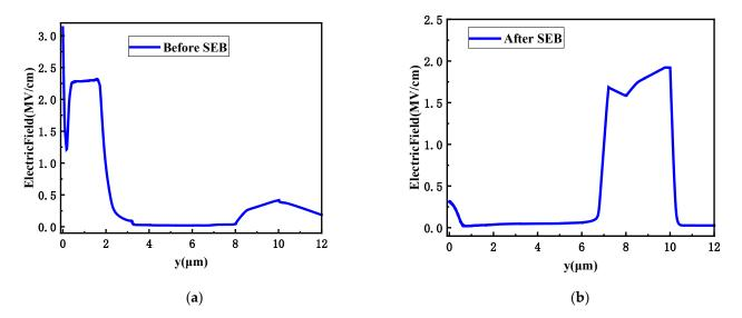
**Figure 11.** (a) Electric field distribution before SEB with buffer layer design; (b) Electric field distribution after SEB with buffer layer design.
