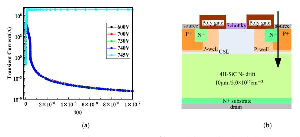
**Figure 8.** (a) Transient current curve of the extended position b in the P+ body contact area; (b) incident position C.
