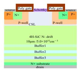
Figure 9. Structure with multi-layer N-type interval buffer layer.
