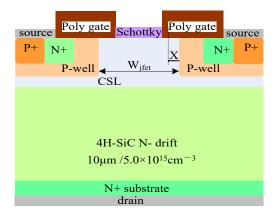
Figure 1. 1200 V SiC MOSFET with split gate and SBD embedded.
