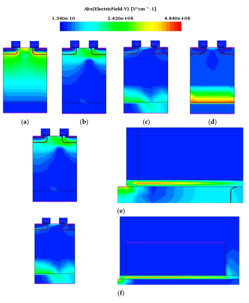
**Figure 6.** Distribution trend of electric field peak transfer during SEB ( $V_{DS} = 450$  V: (**a**) 1 ps; (**b**) 10 ps; (**c**) 100 ps; (**d**)  $10^{-7}$  s; (**e**) enlarged diagram of electric field distribution in the oxide layer at 10 ps; (**f**) enlarged diagram of electric field distribution in the oxide layer at 100 ps.
