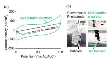
**Figure 4.** Characterization of the microelectrodes for neural stimulation. (**a**) Electric double layer capacitance measured by cyclic voltammetry in a physiological saline solution at scanning speed 20 mV/s from 0 V to 0.8 V vs. Ag/AgCl. Photographs of (**b**) conventional Pt electrode and CNT/paraffin electrode under electrical stimulation at 10 V in a physiological saline.
