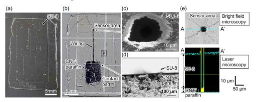
**Figure 2.** Photographs of (**a**) the SU-8 template mold and (**b**) printed CNT/paraffin electrode with SU-8 insulation layer on top with locally exposed sensor area. SEM images of (**c**) the sensor area and (**d**) the boundary between the SU-8 insulation layer and CNT/paraffin contact pad. (**e**) A bright field microscopic image (**top**) and laser microscopic cross-sectional view (**bottom**) of the sensor area.
