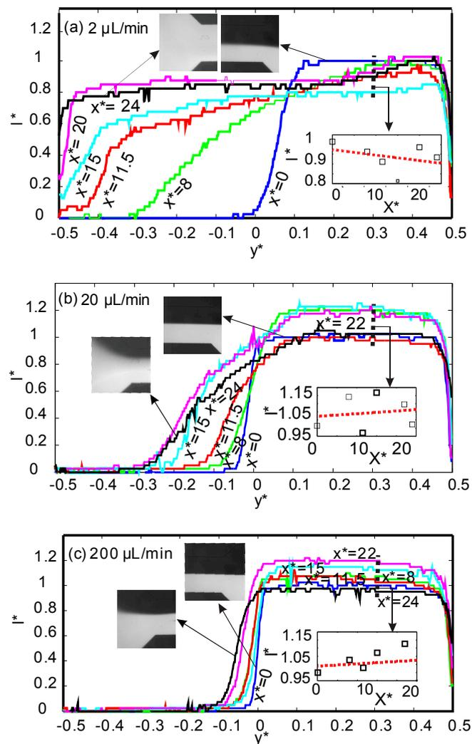
**Figure 2.** Normalized intensity across the normalised channel width  $y^*$  for six positions of  $x^*$  along the mixing channel with a ferrofluid concentration of 2% vol. ( $x^* = 0$ : blue,  $x^* = 8$ : green,  $x^* = 11.5$ : red,  $x^* = 15$ : cyan,  $x^* = 22$ : purple,  $x^* = 24$ : black) and three flow different flow rates: (a) 2  $\mu\text{L}/\text{min}$ ; (b) 20  $\mu\text{L}/\text{min}$ ; (c) 200  $\mu\text{L}/\text{min}$ .
