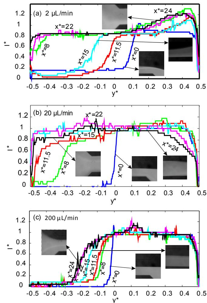
**Figure 3.** Normalized intensity across the normalized channel width  $y^*$  for six positions of  $x^*$  along the mixing channel with a ferrofluid concentration of 20% vol. ( $x^* = 0$ : blue,  $x^* = 8$ : green,  $x^* = 11.5$ : red,  $x^* = 15$ : cyan,  $x^* = 22$ : purple,  $x^* = 24$ : black) and three different flow rates: (a)  $2 \mu\text{L}/\text{min}$ ; (b)  $20 \mu\text{L}/\text{min}$ ; (c)  $200 \mu\text{L}/\text{min}$ .
