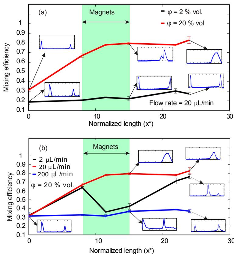
**Figure 4.** Mixing efficiency along the normalized channel length  $x^*$  with probability distribution graphs of selected points: (a) Constant flow rate of  $20\ \mu\text{L}/\text{min}$  and ferrofluid concentrations of 2 and 20% vol.; (b) Constant concentration of 20% vol. and three flow rates of 2, 20, and  $200\ \mu\text{L}/\text{min}$ .
