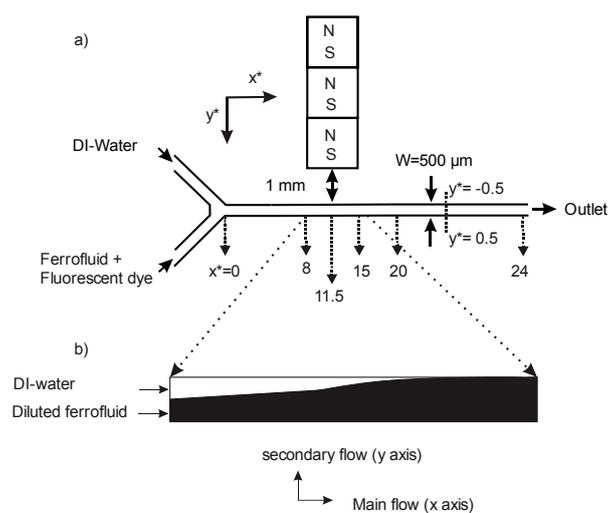
**Figure 1.** Schematic of the experiment (a) Experimental setup ( $x^* = x/W$ ,  $y^* = y/H$ ); (b) Deflection of superparamagnetic ferrofluid stream towards the magnets due to magnetoconvection, based on experimental observation.
