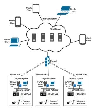
Figure 2. Architecture of cloud-based SCADA systems (inspired by [15]).
