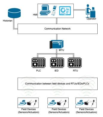
Figure 1. Architecture of traditional SCADA systems (inspired by [2]).
