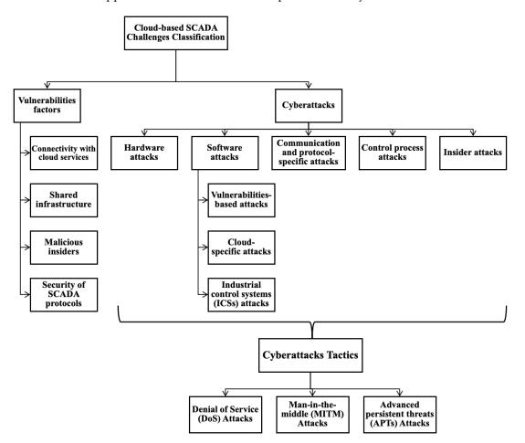
Figure 3. Classification of the security challenges of cloud-based SCADA systems.
