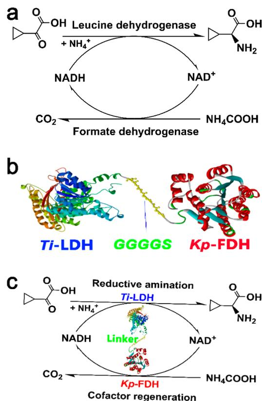
**Figure 2.** (a) Enzyme-coupled biocatalytic process for the synthesis of (*S*)-2-cyclopropylglycine and cofactor regeneration. (b) Construction of bifunctional enzyme, and (c) Bifunctional enzyme-mediated asymmetric synthesis of (*S*)-2-cyclopropylglycine and cofactor regeneration.
