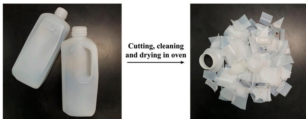
**Figure 1.** HDPE milk bottles and rHDPE obtained after cutting, cleaning and drying.
