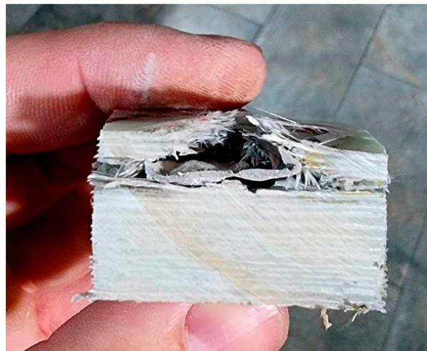
**Figure 11.** The cut sample for SEM investigation (after test with 0.357 Magnum).
