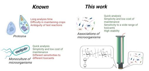
Figure 1. The biosensor formation approach used in this study.
