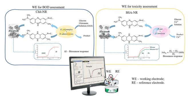
**Figure 6.** BOD toxicity biosensor design. Insert: the current increasing is associated with the adding of a model solution into the system (GGS for BOD analysis, Glucose and  $Cu^{2+}$  solution is for toxicity analysis). For the water sample BOD assessment, the GGS solution is replaced with the sample. For toxicity assessment,  $Cu^{2+}$  is replaced with the sample (glucose was diluted in the sample at the same concentration for the control solution test).
