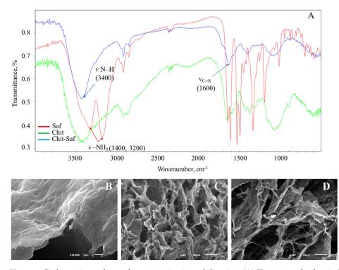
**Figure 8.** Redox-active polymer for association immobilization. (**A**) IR spectra of safranin O, chitosan, and a redox-active polymer, where  $v - NH_2$  are stretching vibrations of  $-NH_2$ , v C=N are stretching vibrations of C=N. (**B**) SEM images of BSA-FC-CNT/COOH nanocomposite. (**C**) SEM images of CHIT-FC redox-active polymer. (**D**) SEM images of BSA-FC redox-active polymer.
