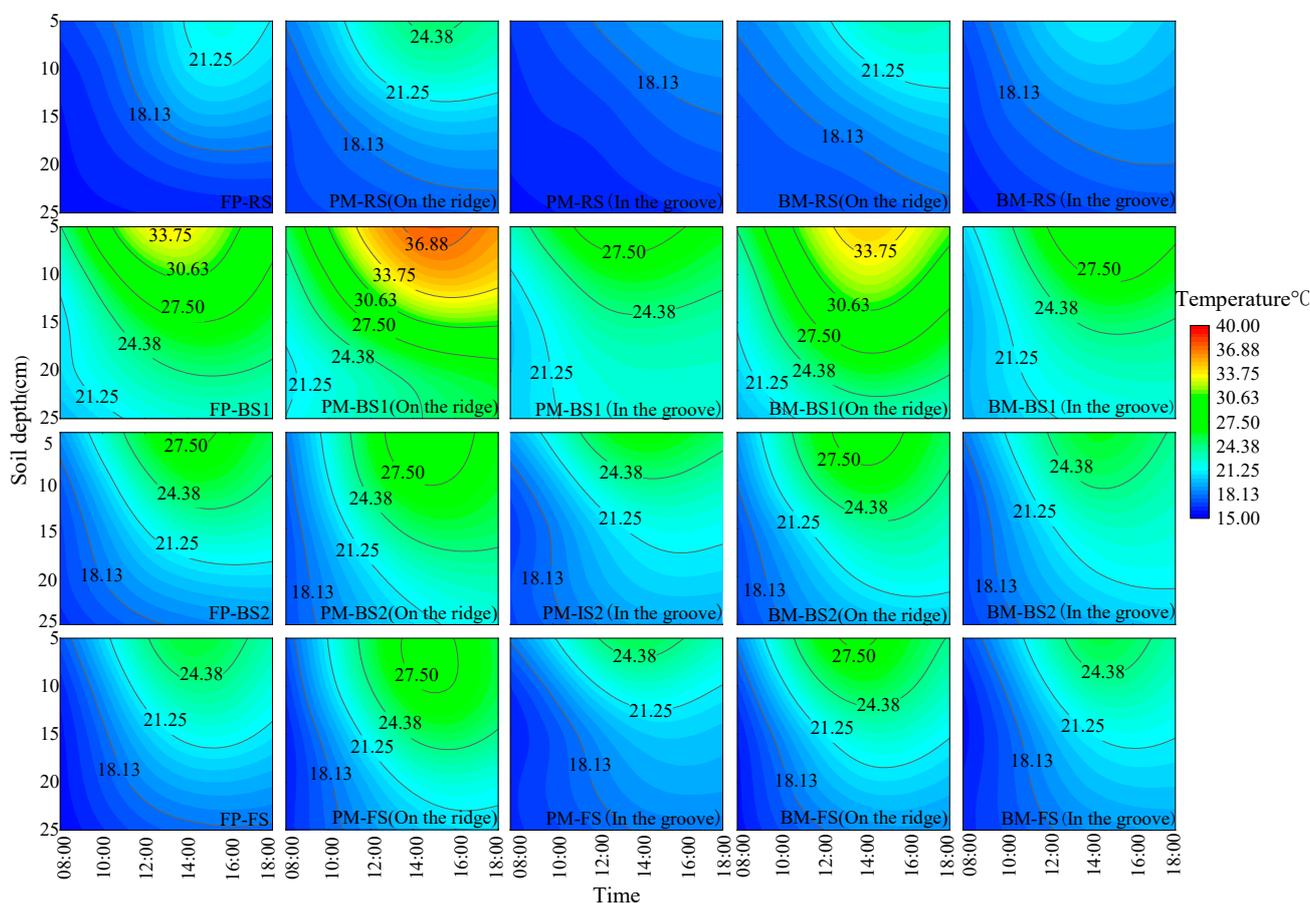
**Figure 4.** Temporal and spatial changes of lucerne soil temperature under different planting patterns. In the figure, regreening stage, branching stage, initiation of flowering stage and flowering stage were used respectively as RS, BS1, BS2, and FS. PM, BM, and FP represent ridge mulching with ordinary plastic film, ridge mulching with biodegradable film, and traditional flat planting, respectively.
