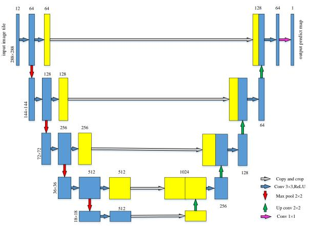
Figure 2. UNET structure.
