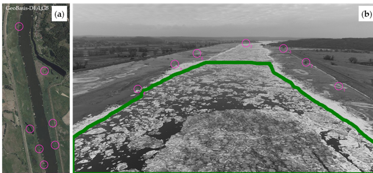
Figure 8. Representation of selected processing steps within the PTV workflow. Pink circles represent ground control points. (a) Orthophoto of the investigation area of the Oder River. (b) Processed UAV image with delineation of the area of interest (green frame).
