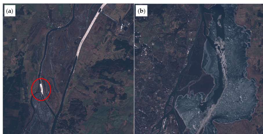
Figure 16. (a) Ice displacement on the West Oder (red circle) discovered using Sentinel-2 image supporting ice-breakup operations during the 2021 ice-jam event. (b) Sentinel-2 image showing ice floe transport channel on Dabie Lake on 22 February 2021.
