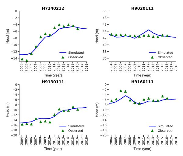
Figure 6. The simulated variation and observation data of groundwater level at four boreholes.
