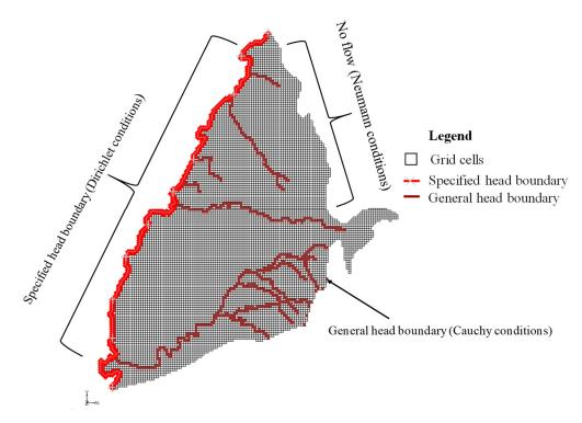
Figure 3. Boundary conditions set-up in MODFLOW model.
