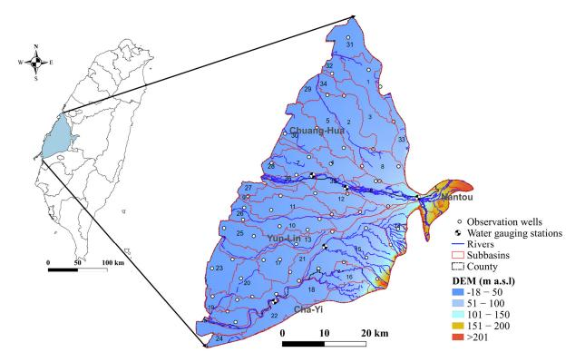
**Figure 1.** Location of the Choushui River Alluvial Fan and the delineation in SWAT and MODFLOW. Numerical identifiers in the figure correspond to each sub-basin.
