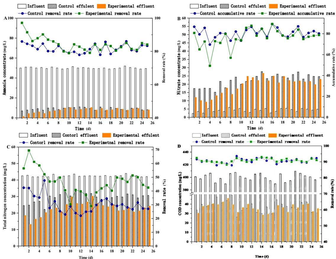
**Figure 2.** Characteristics of (A) ammonium, (B) nitrate, (C) total nitrogen and (D) COD in the MBR systems.
