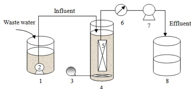
**Figure 1.** Schematic diagram of the MBR reactor. (1) Influent tank; (2) submersible pump; (3) aerator; (4) MBR; (5) membrane module; (6) pressure gauge (7) peristaltic pump; (8) effluent tank.
