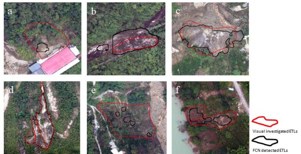
Figure 8. The type of automatic detection errors. (a) The landslide detection area in black line is smaller than the actual area in red. (b) The landslide detection area is larger than the actual area. (c) The detected area of the landslide partially coincides with the actual area. (d) A landslide is detected as multiple landslides. (e) Multiple landslides are detected as a single landslide. (f) Multiple landslides are detected as multiple landslides.
