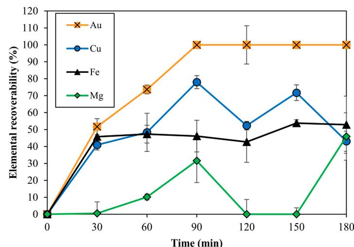
**Figure 14.** The elemental recovery by electrowinning (EW) from the diluted aqua-regia containing gold (initial pH 2.00); data are presented as the mean  $\pm$  SD ( $n = 3$ ).
