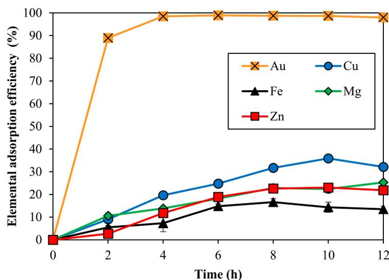
**Figure 11.** The elemental adsorption efficiency from the second leachate using activated carbon; data are presented as the mean  $\pm$  SD ( $n = 3$ ).
