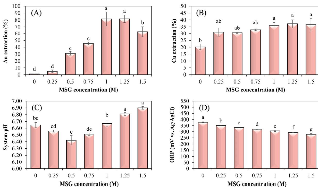
**Figure 6.** Effect of MSG concentration on gold leaching (A), copper leaching (B), system pH (C), and ORP (D) from the solder-mask-free WPCB residue (obtained from the first leaching using 0.75 M MSG supplemented with 1% (*w/v*)  $H_2O_2$  at 4% pulp density) using a fresh 1% (*w/v*)  $H_2O_2$  as an oxidizer at 4% (*w/v*) pulp density for 3 h; different lowercase letters on the bars indicate significant differences ( $p < 0.05$ ); data are presented as the mean  $\pm$  SD ( $n = 3$ ).
