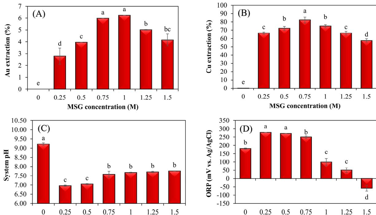
**Figure 5.** Effect of MSG concentration on gold leaching (A), copper leaching (B), system pH (C), and ORP (D) from solder-mask-free WPCBs using 1% (*w/v*) H<sub>2</sub>O<sub>2</sub> as an oxidizer at 4% (*w/v*) pulp density for 3 h; different lowercase letters on the bars indicate significant differences ( $p < 0.05$ ); data are presented as the mean  $\pm$  SD ( $n = 3$ ).
