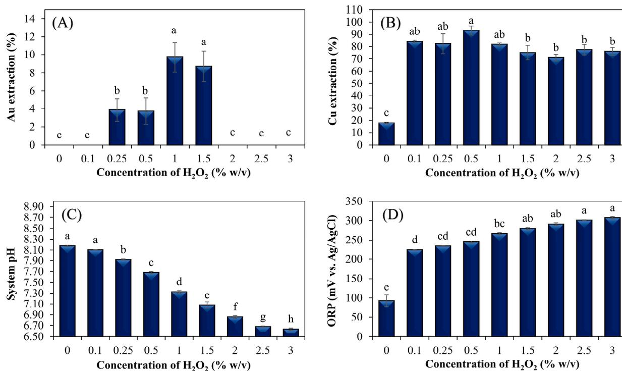
**Figure 7.** Effect of H<sub>2</sub>O<sub>2</sub> concentration on gold leaching (A), copper leaching (B), system pH (C), and ORP (D) from solder-mask-free WPCBs using 0.75 M MSG as a chelator at 4% (w/v) pulp density for 3 h; different lowercase letters on the bars indicate significant differences ( $p < 0.05$ ); data are presented as the mean  $\pm$  SD ( $n = 3$ ).
