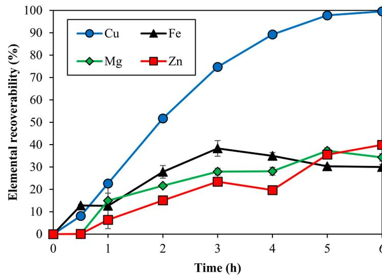
**Figure 10.** The recoverability of metals in the first leachate using electrowinning (EW); data are presented as the mean ± SD (n = 3).
