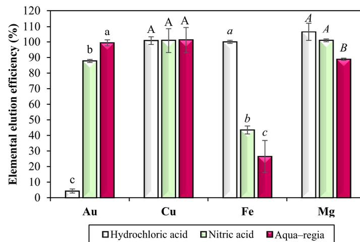
**Figure 13.** The elution efficiency of metals from the pre-eluted gold-loaded activated carbon; the lowercase letters, the capital letters, the italic lowercase letters, and italic capital letters on the bars indicate significant differences ( $p < 0.05$ ) in the elution efficiencies of gold, copper, iron, and magnesium for each treatment, respectively; data are presented as the mean  $\pm$  SD ( $n = 3$ ).
