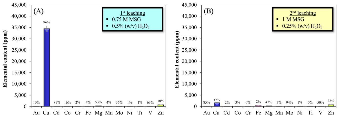
**Figure 9.** The extracted elements under optimal conditions from solder-mask-free WPCBs (A) and solid residues (B) in the leachate of the first leaching (0.75 M MSG, 0.5% (w/v) H<sub>2</sub>O<sub>2</sub>) and the second leaching (1 M MSG, 0.25% (w/v) H<sub>2</sub>O<sub>2</sub>), respectively; the percentages on the bar represent the extractions (%); data are presented as the mean ± SD (n = 3).
