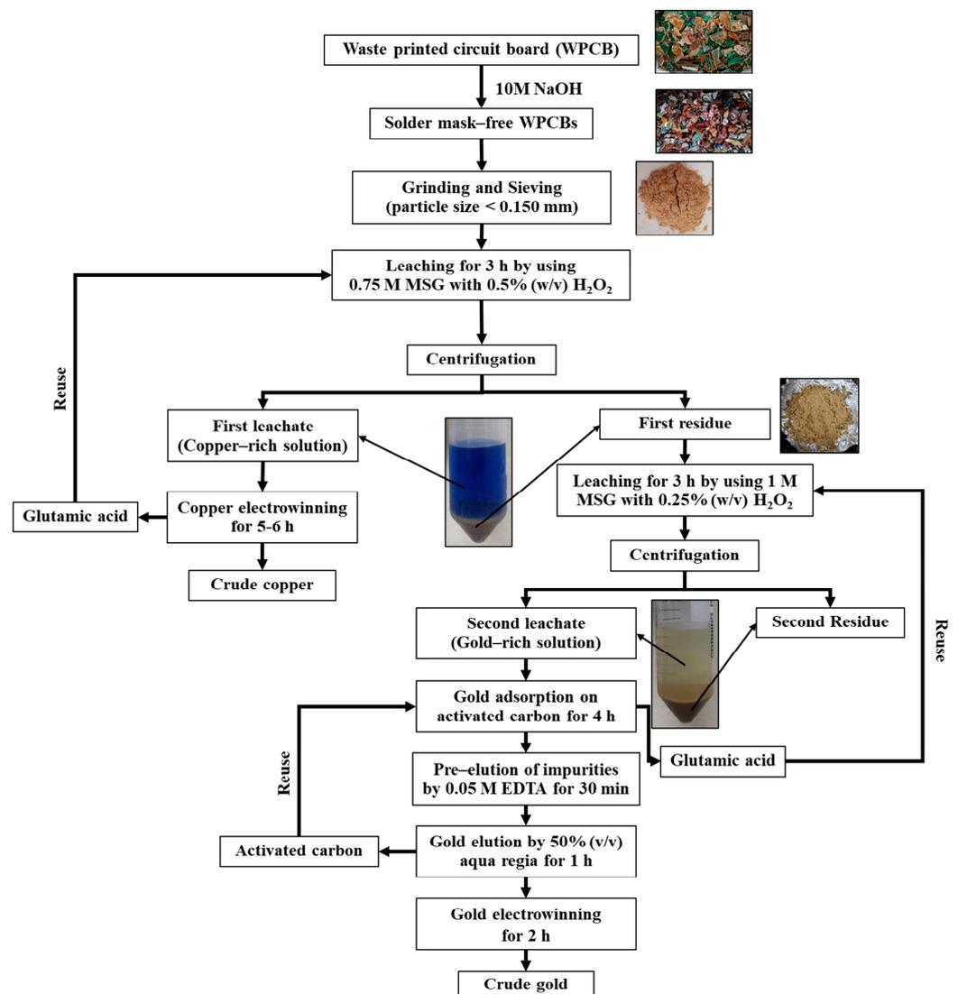
Figure 15. The overall process for recovery of copper and gold from waste printed circuit board.
