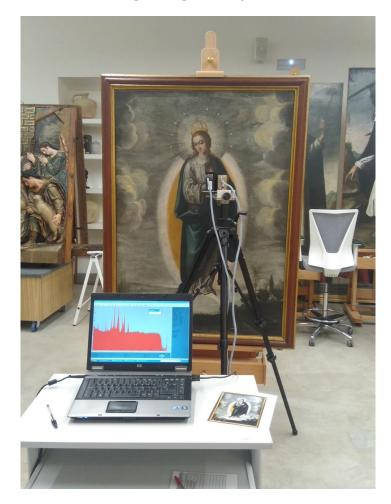
Figure 2. XRF in situ analysis of La Inmaculada.
