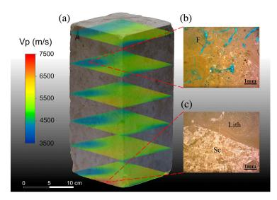
**Figure 13.** Pietra Forte sample: integrated analysis of ultrasonic tomography and thin sections. (a) Tomography horizontal slices incorporated within the 3D HR CRP model. (b) Microscopic features of a porous sector of the sample; OM plane polarized light; thin section treated with blue dye epoxy resin. F (fracture secondary porosity). (c) Microscopic features of a compact sector of the sample; OM cross polarized light. Lith (Lithothamnium algae); Sc (sparry calcite).
