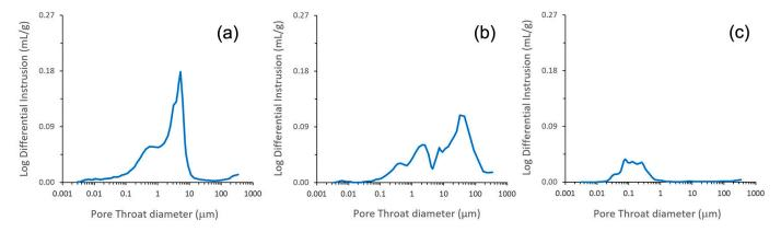
**Figure 5.** MIP curves highlighting the pore-throat size distributions of three representative samples of the Calcari di Cagliari: (a) Pietra Cantone; (b) Tramezzario; (c) Pietra Forte.
