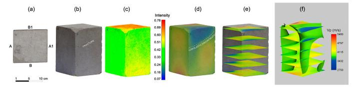
**Figure 10.** Results of the 3D analyses by the integrated approach for the Tramezzario sample. (a) Localization of the different faces of the sample; (b) 3D HR CRP model texturized with natural colors and represented in a RGB scale; (c) 3D HR CRP model texturized with the intensity of ambient light; (d) 3D ultrasonic tomography incorporated within the 3D HR CRP model; (e) Tomography horizontal slices; (f) Isosurface of 3800 m/s with the horizontal slices.
