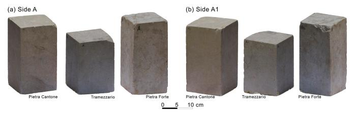
**Figure 6.** (a) Side A view of the HR 3D models of the three prismatic samples under study texturized with natural colors. (b) Side A1 view.
