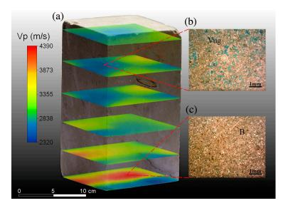
**Figure 9.** Pietra Cantone sample: integrated analysis of ultrasonic tomography and thin sections. (a) Tomography horizontal slices incorporated within the 3D HR CRP model. (b) Microscopic features of a porous sector of the sample; OM plane polarized light; thin section treated with blue dye epoxy resin. Vug (vug secondary porosity). (c) Microscopic features of a compact sector of the sample; OM cross polarized light. B (bioclast).
