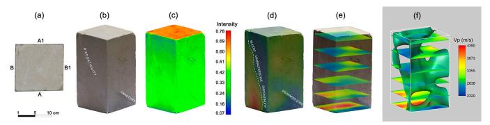
**Figure 8.** Results of the 3D analyses by the integrated approach for the Pietra Cantone sample. (a) Localization of the different faces of the sample. (b) 3D HR CRP model texturized with natural colors and represented with an RGB scale. (c) 3D HR CRP model texturized with the intensity of ambient light. (d) 3D ultrasonic tomography incorporated within the 3D HR CRP model. (e) Tomography horizontal slices. (f) Isosurface of 2800 m/s with horizontal slices.
