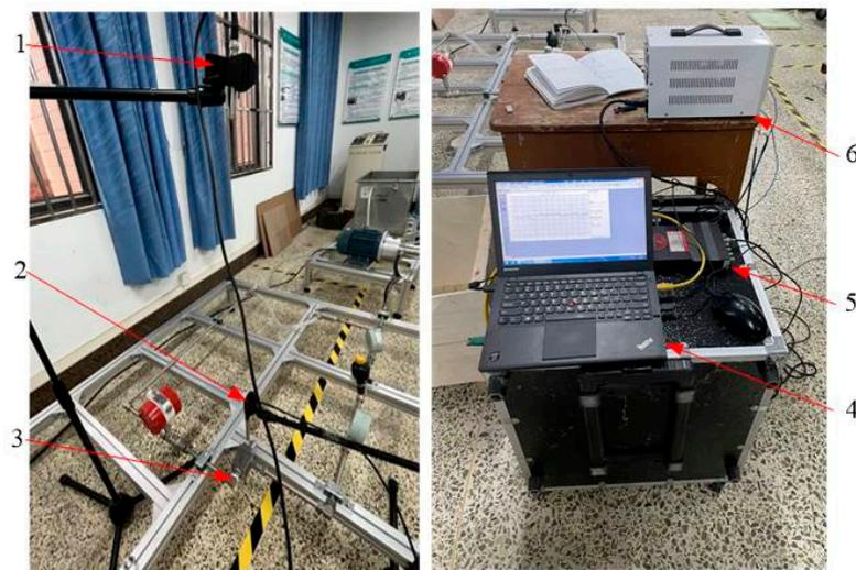
**Figure 14.** The water hydraulic throttle valve noise experimental bench. 1—microphone 1, 2—microphone 2, 3—water hydraulic throttle valve, 4—the acquisition system, 5—computer, 6—DC power supply.
