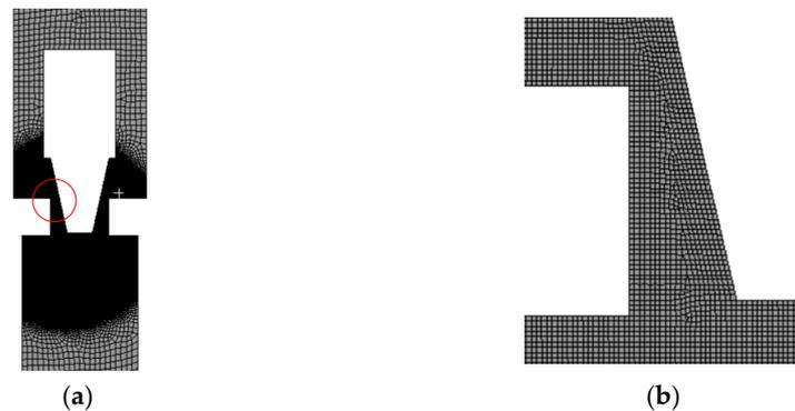
**Figure 2.** Mesh of the throttle valve: (a) The mesh of the throttle valve; (b) mesh local magnification.
