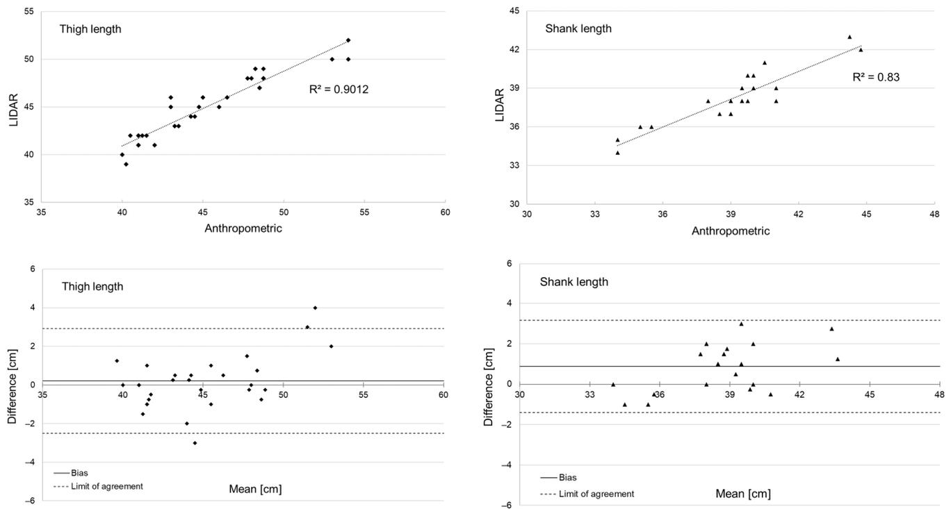
**Figure 2.** Correlation (**top**) with coefficient of determination ( $R^2$ ) and Bland–Altman plots (**bottom**) with the confidence interval at 95% limits of agreement between LiDAR-based and manual anthropometric measures of thigh length (**left**) and shank length (**right**). Length measures from the left and right leg of each participant (i.e.,  $n = 16$  thigh,  $n = 11$  shank) were taken into account.
