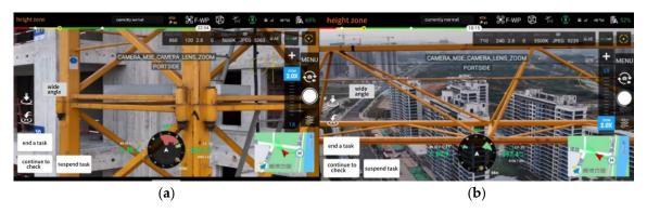
**Figure 9.** Operating interface of the UAV intelligent inspection application. (a) Automated shooting of the standard sections by UAV. (b) Automated shooting of the tower crane boom by UAV.
