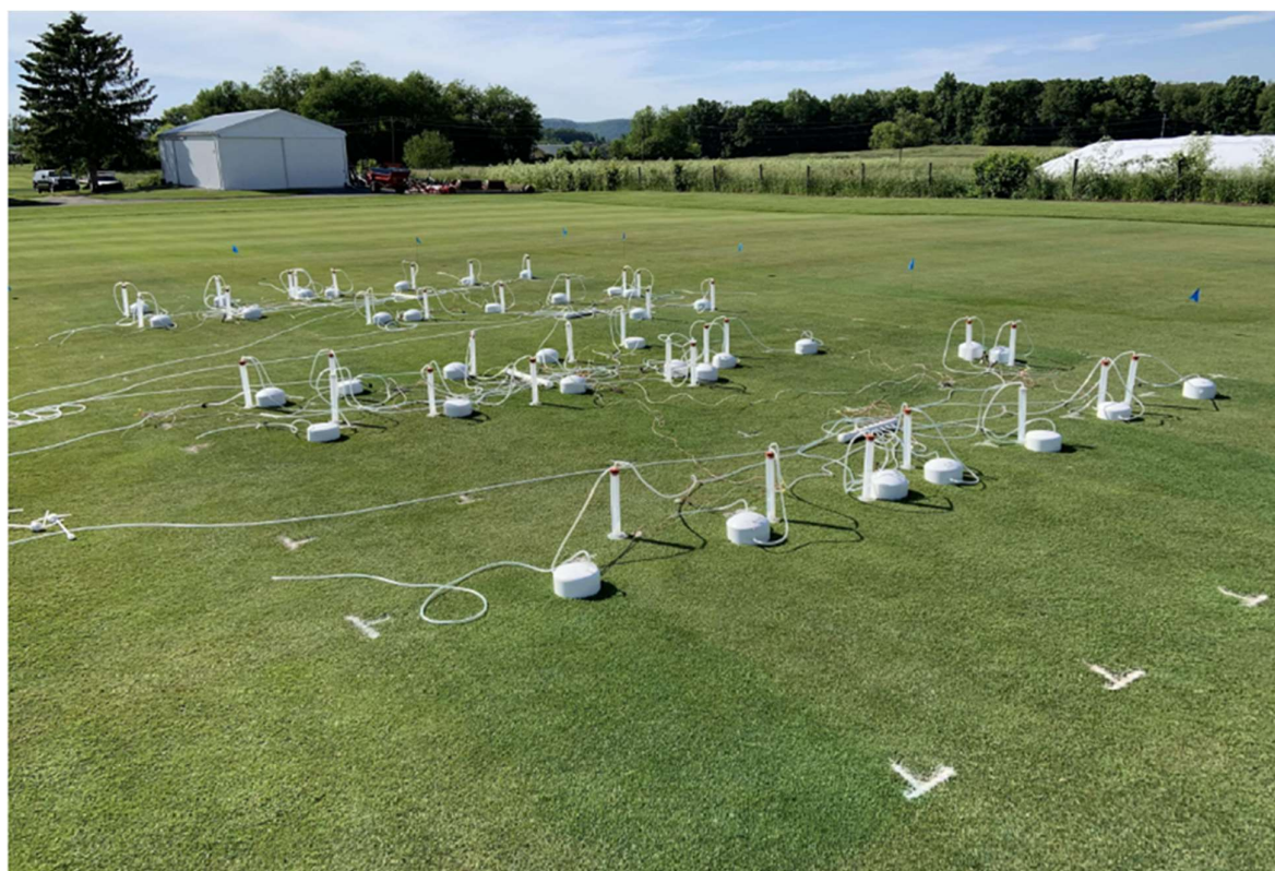
Figure 1. Experimental plots equipped with closed flux chambers and boric acid scrubbing flasks facilitating the in situ measurement of ammonia emission, 9 June 2020 (Valentine Turfgrass Research Center, University Park, PA).
