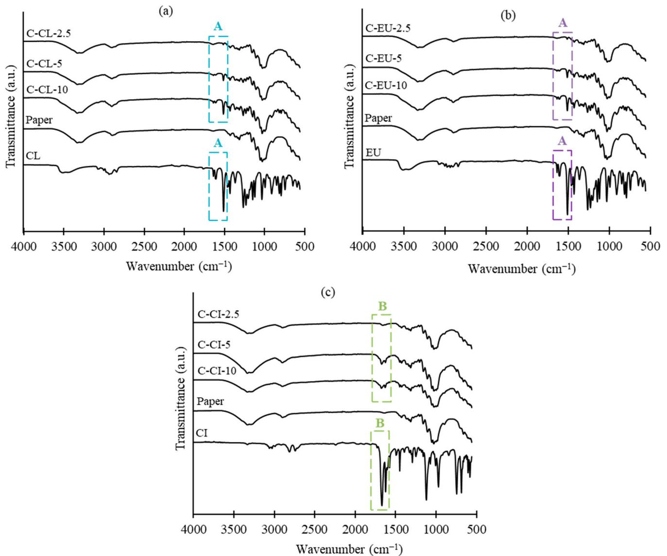
**Figure 5.** FT-IR spectra of samples: (a) clove essential oil (CL), paper and coated paper sheets (C-CL); (b) eugenol (EU), paper and coated paper sheets (C-EU); (c) cinnamaldehyde (CI), paper and coated paper sheets (C-CI). The dashed line boxes and letters show the groups of the absorption peaks: A—1636, 1607, and 1512  $\text{cm}^{-1}$ ; B—1670  $\text{cm}^{-1}$ .
