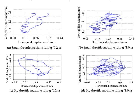
Figure 11. Axis locus of threshing cylinder under 200 g counterweight condition.
