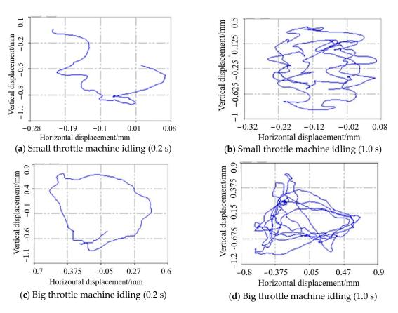
**Figure 17.** Track of threshing cylinder axis under the condition of 200 g top cover, 200 g concave plate screen, and 200 g balance weight between the top cover and concave plate screen.
