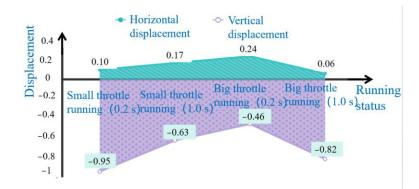
**Figure 16.** Displacement change in threshing drum under the top cover of 200 g and concave screen of 200 g.
