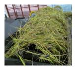
Figure 5. A winding stalk on a threshing drum.
