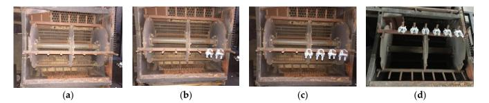
**Figure 8.** Tests to explore the distribution of eccentric mass along the axial direction. (**a**) No additional counterweight; (**b**) Add 200 g of breeding blocks; (**c**) Add 400 g of counterweight; (**d**) Add 600 g of counterweight.
