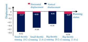
Figure 14. Displacement change in threshing drum under 600 g counterweight condition.
