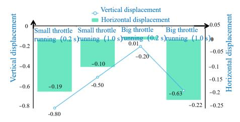
**Figure 18.** Displacement change in threshing drum with 200 g top cover, 200 g concave screen, and 200 g counterweight between the top cover and concave screen.
