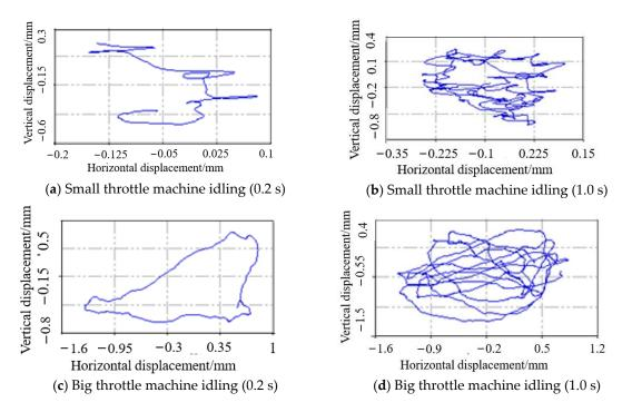
Figure 10. Axis locus of threshing cylinder without counterweight.
