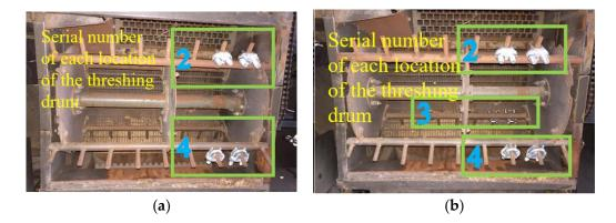
**Figure 9.** Tests to explore the radial distribution of eccentric mass. (**a**) Add 400 g counterweight (top cover 200 g, concave screen 200 g); (**b**) Add 600 g counterweight (200 g for top cover, 200 g for concave screen, 200 g between the top cover and concave screen).
