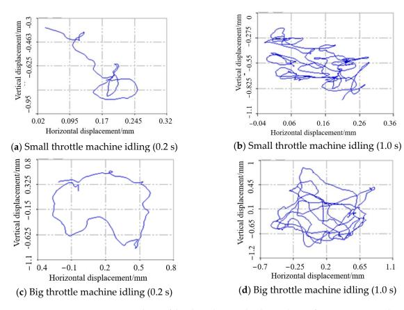
**Figure 15.** Axis locus of threshing drum under the condition of top cover 200 g and concave screen 200 g counterweight.
