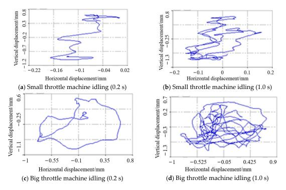
Figure 12. Axis locus of threshing cylinder under 400 g counterweight condition.
