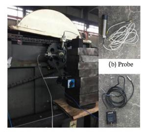
(a) Eddy current sensor field layout (c) Preprocessor
