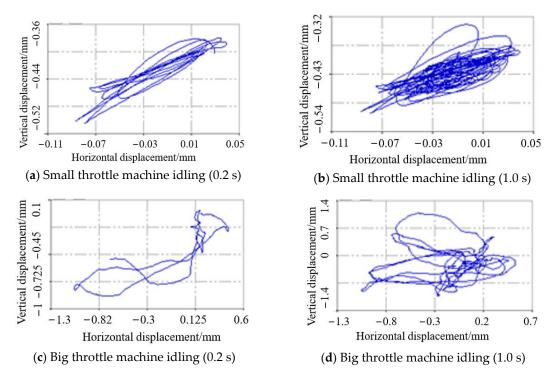
Figure 13. Axis locus of threshing cylinder under 600 g counterweight condition.
