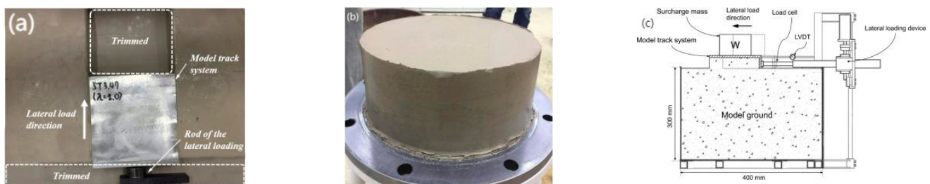
Figure 14. (a) Trimmed model ground; (b) reconstituted EPK kaolinite specimen; (c) schematic diagram of the model track experiments [67].
