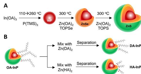
**Scheme 1.** (A) The preparation of the InP cores and growth of the ZnSe/ZnS shell. (B) The ligand exchange process.
