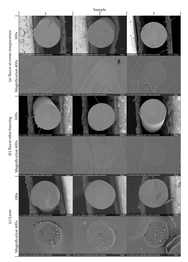
Figure 4. Cross-sectional SEM images of the three cutting methods; (a) razor at room temperature, (b) razor after freezing, and (c) laser.
