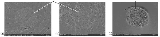
**Figure 12.** Direct comparison of razor and laser-cut samples; (**a**) razor at room temperature, (**b**) razor after freezing, and (**c**) laser.
