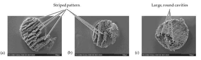
**Figure 13.** Comparison of surface pattern with varied laser power at 5 mm/s; (**a**) 20 W, (**b**) 60 W, and (**c**) 100 W.
