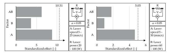
Figure 11. Pareto charts of standardized effects of linear resistivity and laser parameters.
