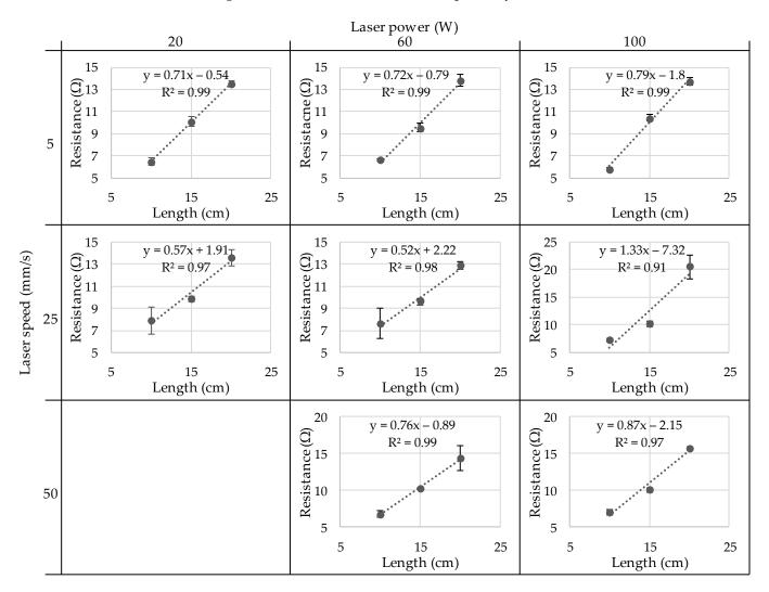
Figure 7. Linear dependence of resistance and sample length.
