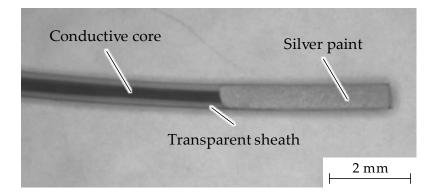
Figure 3. Image of a cut and silver painted bicomponent filament.
