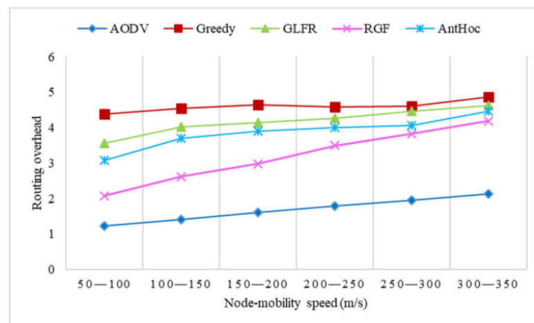
Figure 16. The effect of velocity on routing overhead.
