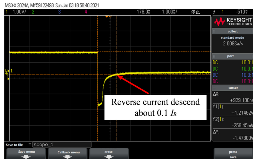
Figure 15. Test results of reverse recovery time t_r .
