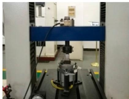
**Figure 2.** The stiffness testing of the electro-hydraulic engine mounts.
