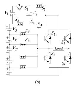
**Figure 1.** Proposed topology: (a) proposed circuit–I topology; (b) generalized proposed circuit–I topology.
