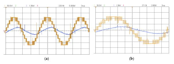
Figure 14. Load voltage and current for the 9-level inverter: (a) 2.5 cycles; (b) 1 cycle.
