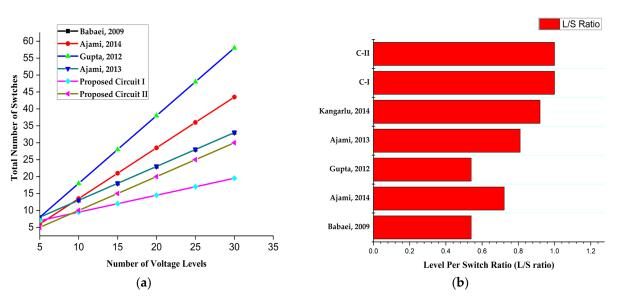
**Figure 8.** Comparison of the proposed topology with existing topologies in terms of (**a**) total number of switches required for different voltage level; (**b**) level-per-switch ratio [24–27,29].
