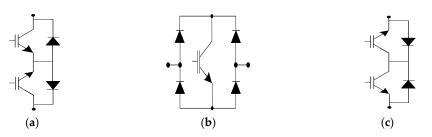
**Figure 3.** Different types of configurations of bi-directional switches (**a**) Common Emitter; IGBT (**b**) Diode Bridge with one Power Switch (**c**) Common Collector IGBT.
