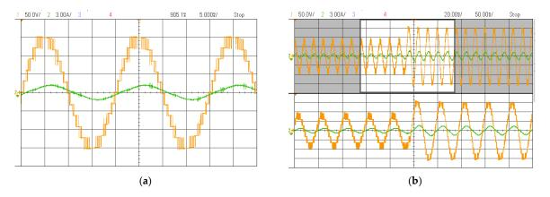
**Figure 16.** Load voltage and current for the 11-level inverter; (**a**) 2.5 cycles; (**b**) different modulation indices.
