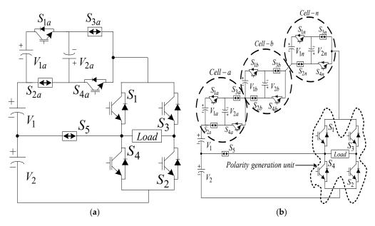
Figure 2. Proposed topology: (a) proposed circuit–II topology; (b) generalized proposed circuit–II topology.
