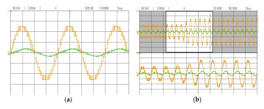
**Figure 17.** Load voltage and current for the 13-level inverter: (**a**) 2.5 cycles; (**b**) different modulation indices.
