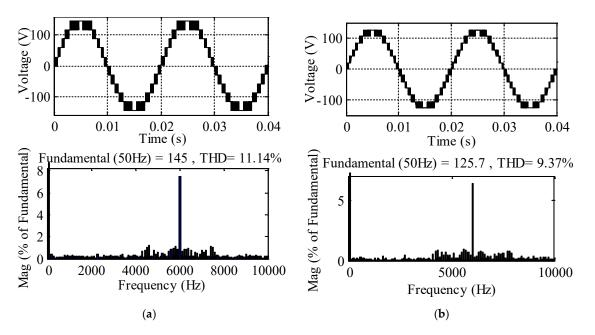
**Figure 15.** Total harmonic distortion of the output voltage of the proposed inverters: (**a**) 11–level inverter; (**b**) 13–level inverter.
