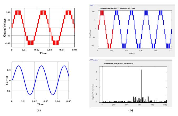
**Figure 12.** Simulation results for the 9-level inverter: (**a**) output voltage and current; (**b**) %THD of output phase voltage.
