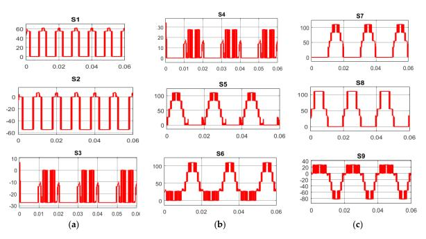
Figure 10. Blocking voltages across the switches: (a) S<sub>1</sub>, S<sub>2</sub>, and S<sub>3</sub>; (b) S<sub>4</sub>, S<sub>5</sub>, and S<sub>6</sub>; (c) S<sub>7</sub>, S<sub>8</sub>, and S<sub>9</sub>.
