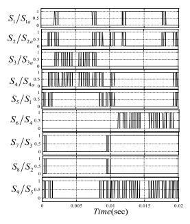
**Figure 6.** Generated pulse pattern for the proposed inverter (circuit–I and circuit–II) for 9-level output voltage.
