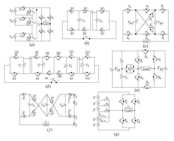
Figure 7. Circuits of the compared topologies proposed in (a) [24]; (b) [25]; (c) [26]; (d) [27]; (e) [28]; (f) [29]; (g) [30].
