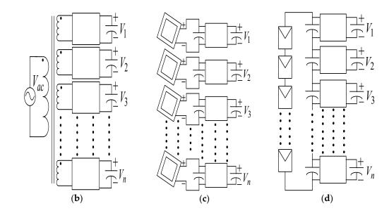
Figure 4. Different ways to generate DC voltages for the capacitors.
