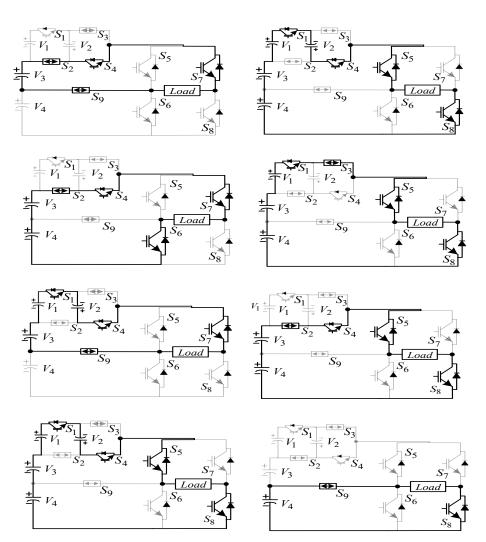
Figure 5. Operating modes for the fundamental structural topology (circuit–I or circuit–II).
