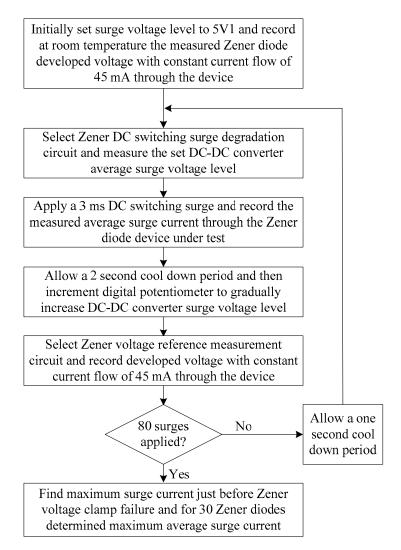
Figure 2. Algorithm flowchart to determine the maximum average surge current level.
