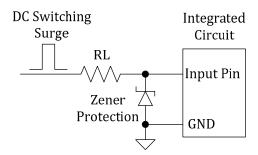
Figure 1. Zener diode DC switching surge protection for IC pins.
