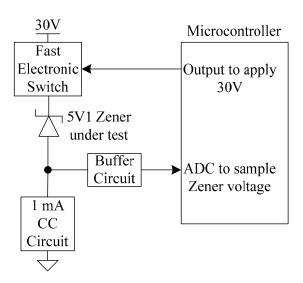
Figure 4. Zener voltage reference measurement circuit.
