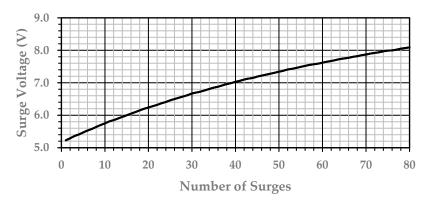
Figure 9. Gradual increasing surge voltage level vs. surge number.
