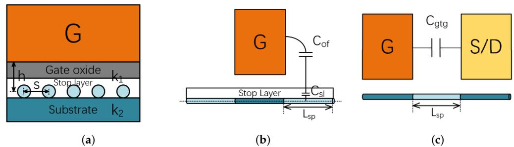
Figure 3. Capacitance structure schematic. (a) Oxide capacitance. (b) Expansion region capacitance. (c) Capacitance between gate and adjacent electrodes.
