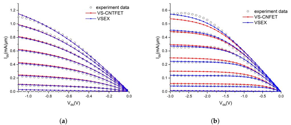
Figure 6. P-type CNTFET output characteristic. (a)  $L_G = 200$  nm; (b)  $L_G = 2$  μm.
