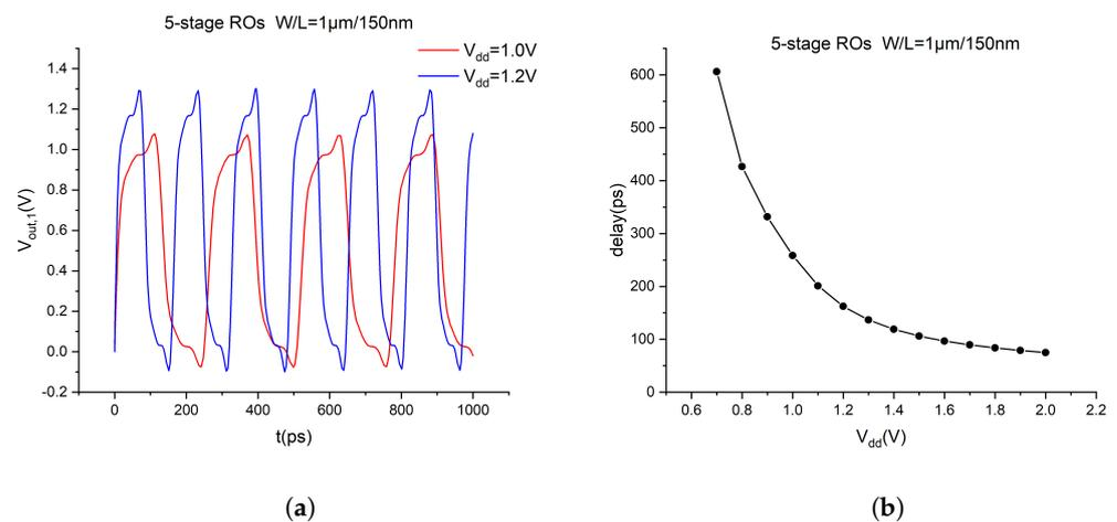
**Figure 9.** 5-stage ring oscillator based on CNTFETs with  $L_G = 150$  nm. (a) Output curves; (b) ro5 delay versus  $V_{dd}$ .
