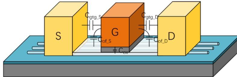
Figure 2. Capacitance in CNTFETs.
