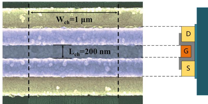
Figure 5. SEM image of the top-view structure of a CNTFET with  $L_G = 200$  nm [6].
