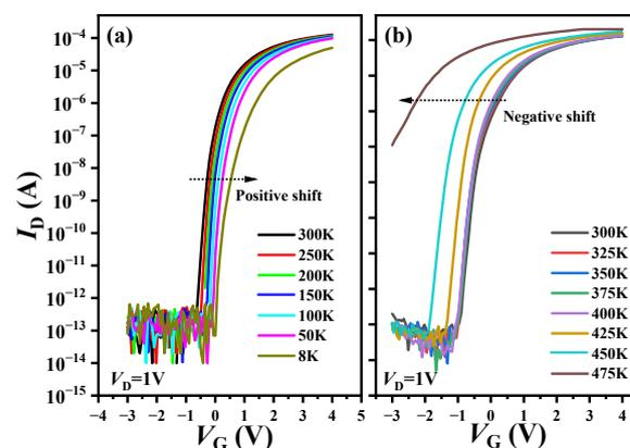
**Figure 2.** (a) The relationship between the  $I_D$ – $V_G$  curve and low-temperature changes. The curve shifts in a positive direction with the temperature decreases. (b) The relationship between the  $I_D$ – $V_G$  curve and high-temperature changes. The curve shifts in a negative direction with the temperature increases.
