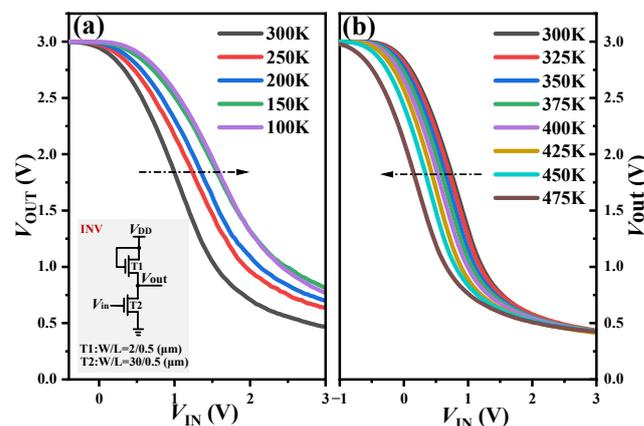
**Figure 9.** (a) The VTC curve of the inverter composed of IGZO TFT varies with low temperature. The inserted diagram is the circuit diagram of the inverter, with T1 as the load transistor and T2 as the drive transistor; (b) the VTC curve of the inverter composed of IGZO TFT varies with high temperature.
