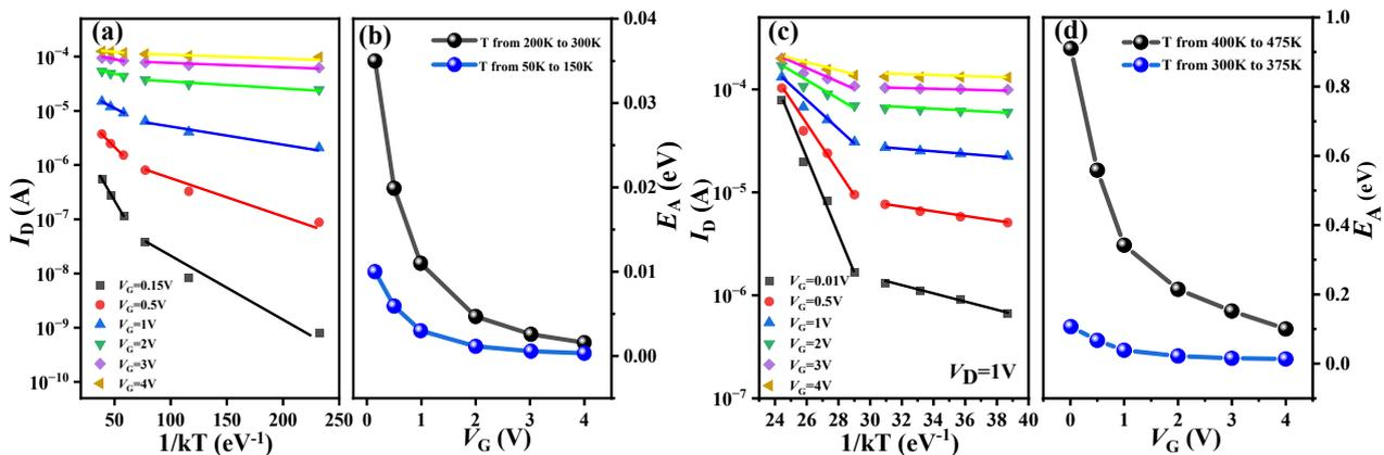
Figure 6. (a) The linear low-temperature dependence between the logarithm of  $I_D$  and  $1/kT$  under different  $V_G$  voltages; lines are used to extract  $E_A$ . (b)  $E_A$  as a function of  $V_G$  within different low-temperature ranges, (c) the linear high-temperature dependence between the logarithm of  $I_D$  and  $1/kT$  under different  $V_G$  voltages. (d)  $E_A$  as a function of  $V_G$  within different high-temperature ranges.
