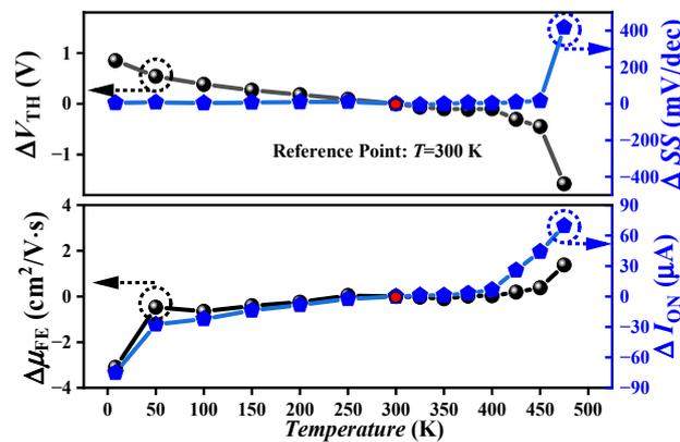
**Figure 3.** Variation of  $\Delta V_{TH}$ ,  $\Delta SS$ ,  $\Delta \mu_{FE}$ , and  $\Delta I_{ON}$  extracted from  $I_D$ - $V_G$  curves with respect to temperature.
