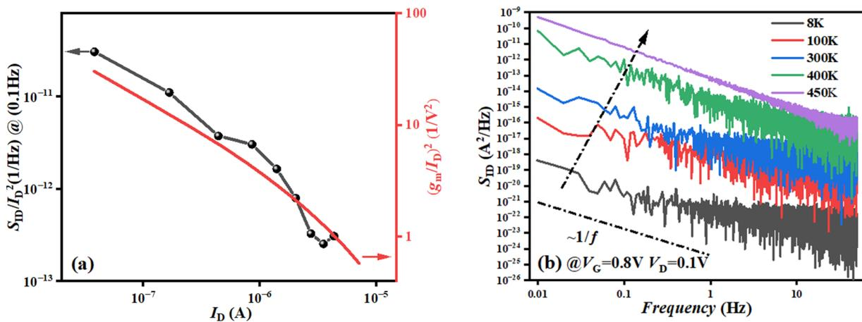
**Figure 8.** (a) The  $S_{ID}/I_D^2$  and the  $(g_m/I_D)^2$  as functions of drain current, in which  $S_{ID}/I_D^2$  follows the trend of  $(g_m/I_D)^2$ ; (b) the relationship between  $S_{ID}$  and frequency at different temperatures, in which  $S_{ID}$  shows an increasing trend with the temperature increases.
