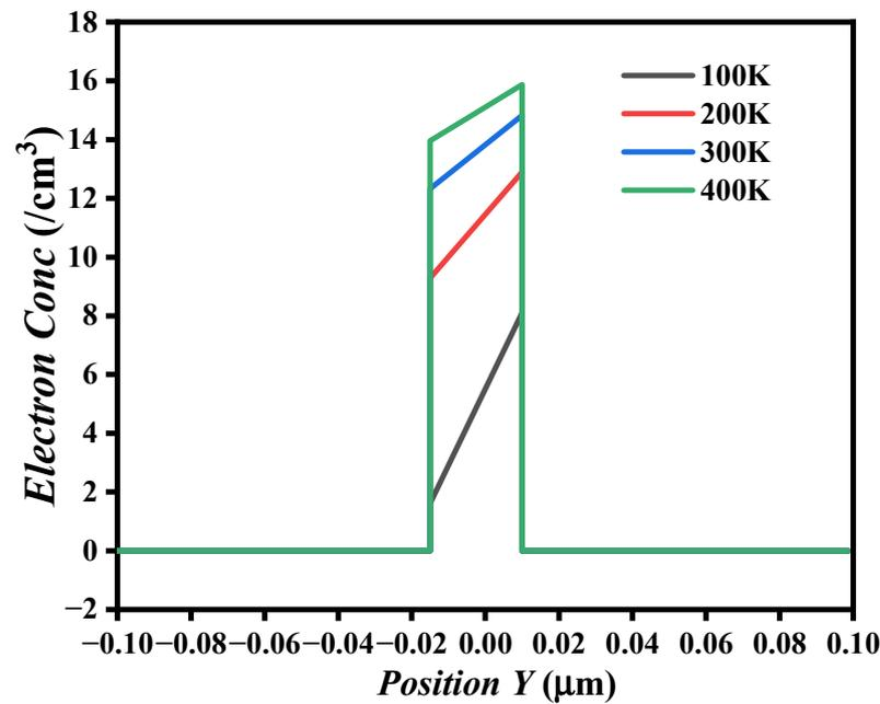
Figure 5. Channel electron concentration variation with temperature for TCAD simulation.
