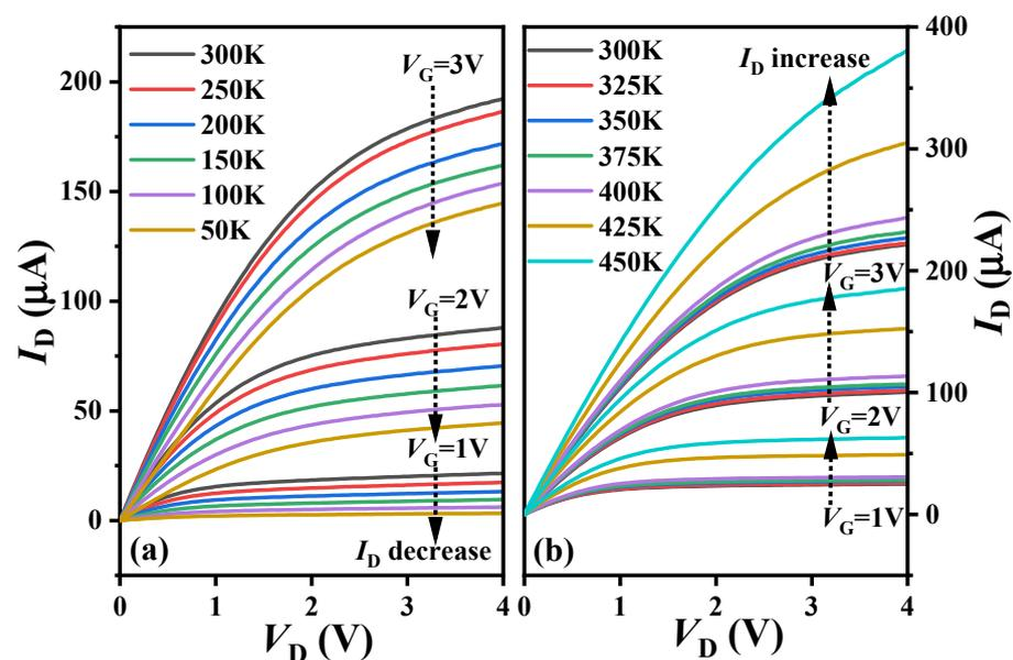
**Figure 4.** (a) The relationship between the  $I_D$ - $V_D$  curve and low-temperature changes. The  $I_D$  decreases with the temperature decreases. (b) The relationship between the  $I_D$ - $V_D$  curve and high-temperature changes. The  $I_D$  increases with the temperature increases.
