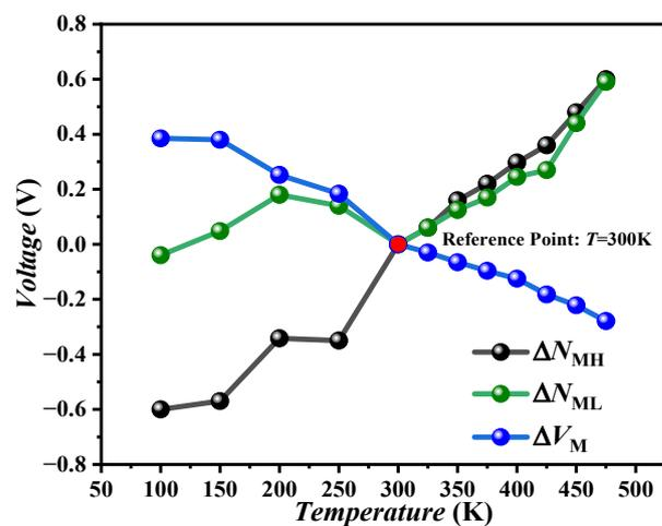
Figure 10. The relationship between the noise margin value of inverters and temperature.
