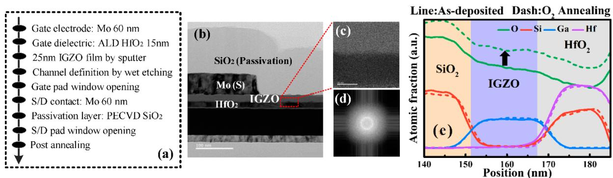
**Figure 1.** (a) Key fabrication process steps for the fabricated back-gated IGZO TFT devices, (b) cross-section TEM image for the IGZO TFT, (c) partial HRTEM image of the interface between the IGZO layer and HfO<sub>2</sub> layer, (d) FFT image, and (e) ESD image for the IGZO TFT.
