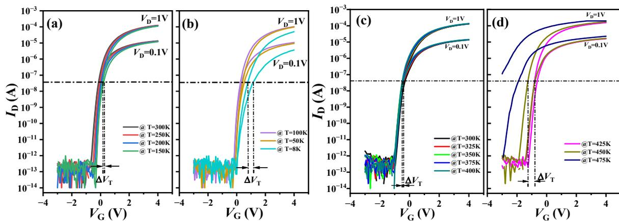
**Figure 7.** (a) Variation of  $I_D$ - $V_G$  curves for IGZO TFT at  $V_D = 0.1$  V and  $V_D = 1$  V within the temperature range of 150–300 K; (b) the DIBL effect of IGZO TFT varies with temperature at extremely low temperature; (c) variation of  $I_D$ - $V_G$  curves for IGZO TFT at  $V_D = 0.1$  V and  $V_D = 1$  V within the temperature range of 300–400 K; (d) the DIBL effect of IGZO TFT varies with temperature at extremely high temperature.
