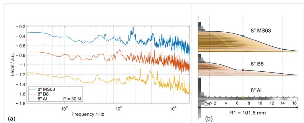
Figure 6. (a) Microphone recorded sound spectra of MS63, B8 cymbals and Al 8-inch, excited by 30 N on the ExP-7. (b) The geometrical characteristics of cymbals with reference to the 8-inch Al sheet.
