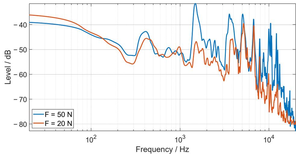
Figure 5. ExP-7 emitted sound spectra excited by 20 N (red line) and 50 N (blue line).
