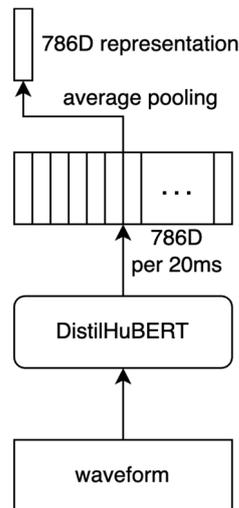
**Figure 3.** Transformation of a waveform in a 768-dimensional representation.
