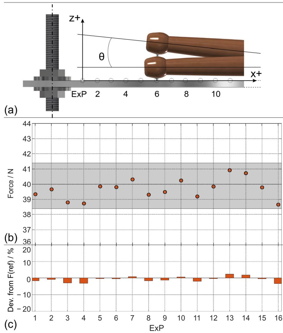
**Figure 2.** (a) The modified drumstick with the hammer tip for  $\theta = 0^\circ$  and  $3^\circ$  at ExP-6 and the axis origin set on ExP-1, (b) mean force for the eight repeated sets of measurements on the 16 ExPs along R1 and (c) deviation % from the reference force  $F = 40$  N.
