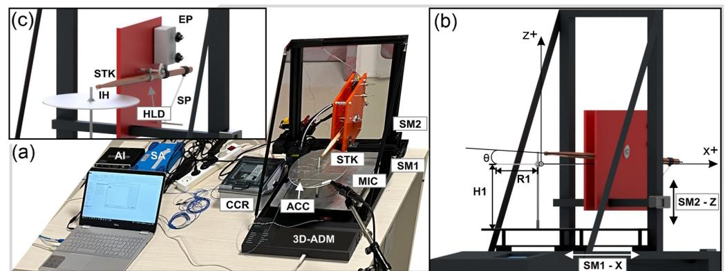
**Figure 1.** The 3D-ADM system generating and collecting the impact sounds: (a) Experimental set-up of the system, (b) CNC spatial adjustment, and (c) Excitation mechanism.
