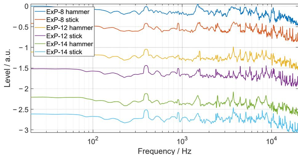
**Figure 4.** Spectra of the emitted sound excited by the modified drumstick with impact force  $F = 40$  N at the representative points ExP-6, -12, and -14 by the hammer vs. the wooden tip (level in a.u.).
