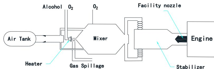
**Figure 1.** Schematic of the incoming flow simulation system.
