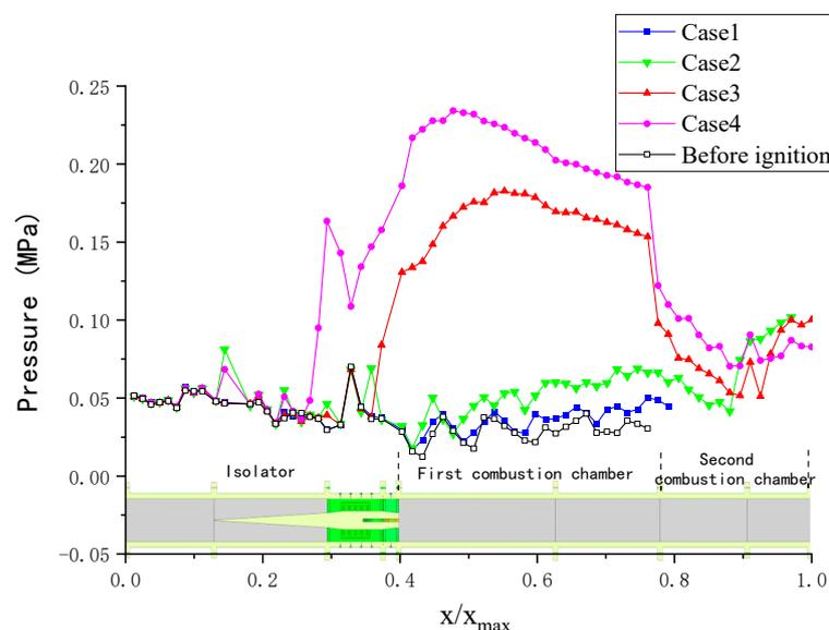
**Figure 8.** The pressure distribution along the wall surface for various equivalence ratios.
