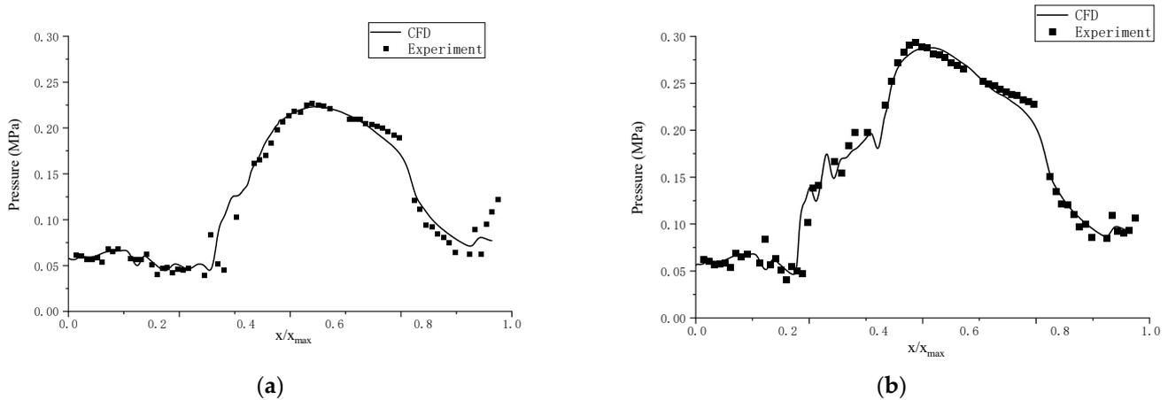
**Figure 10.** Comparison of experimental and numerical pressure distributions along the engine in (a) case 3 and (b) case 4.
