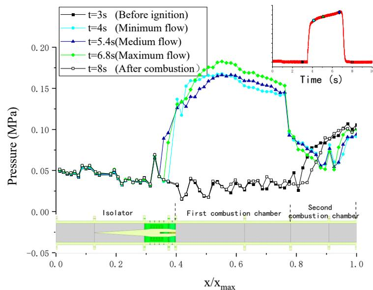
**Figure 7.** The pressure distribution along the wall surface at several moments.
