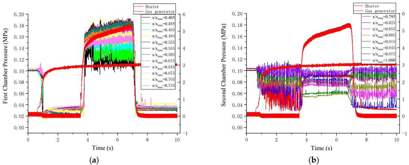
Figure 6. Evolution of wall pressure in case 3 in (a) the first combustor and (b) the second combustor.
