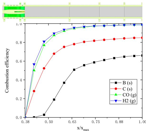
**Figure 11.** Average combustion efficiency in each axial section of combustor.
