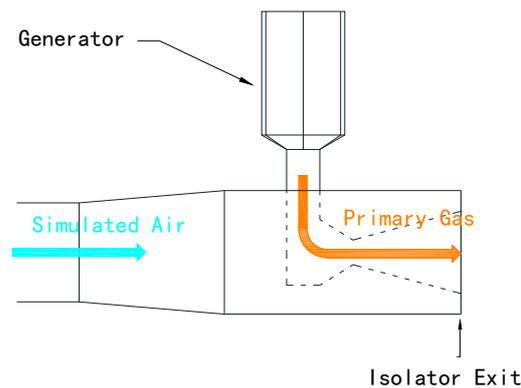
**Figure 3.** Schematic of the central strut injection.
