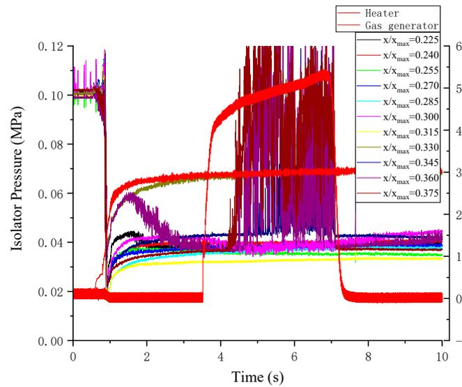
Figure 5. Evolution of wall pressure in the isolator in case 3.
