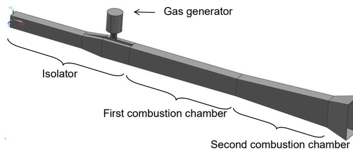
**Figure 2.** Schematic of the solid rocket scramjet.
