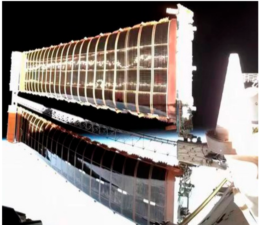
Figure 22. On-orbit state of the flexible solar array.
