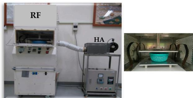
**Figure 1.** Hot air-assisted radio frequency (HARF) equipment (5 kW, 40.68 MHz).
