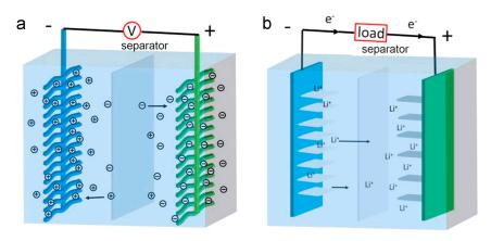
**Figure 7.** Schematic illustrations of energy storage mechanisms of (**a**) a supercapacitor and (**b**) a lithium-ion battery. Reprinted from [95], Copyright 2016, with permission from Elsevier.
