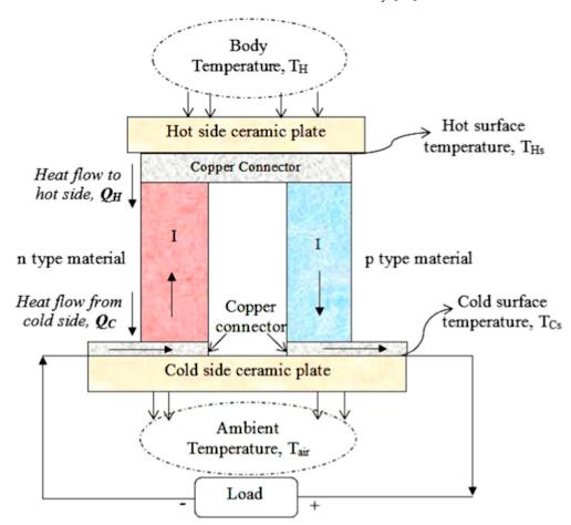
**Figure 4.** Single thermoelectric pair consisting of *n*-type and *p*-type materials. Heat flows from hot side to top side ( $Q_H \rightarrow Q_C$ ), and electrical current (*I*) flows from *n*-type to *p*-type material due to a temperature gradient ( $\Delta T = T_{Hs} - T_{Cs}$ ). Reprinted from [75], Copyright 2017, with permission from Elsevier.
