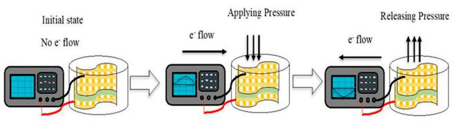
**Figure 6.** Working principle of a piezoelectric material when applying and releasing pressure. Reprinted from [85], originally published under a CC-BY license.
