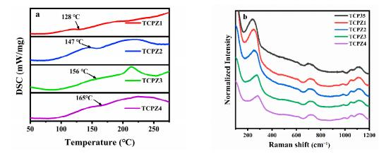
Figure 4. DSC curves (a) and Raman spectra (b) of TCPZ glasses.
