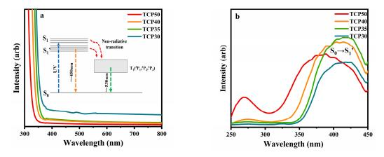
**Figure 1.** (a) Absorption spectra of TCP glasses, inset: Sn<sup>2+</sup> energy transfer model; (b) PLE spectra of TCP glasses under 530 nm excitation.
