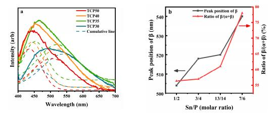
**Figure 2.** (a) PL spectra of TCP glasses. Two emission peaks obtained by Gaussian fitting are marked: (b) Peak area ratio  $\beta/(\alpha + \beta)$  and peak position in the  $\beta$ -band as a function of the P/Sn ratio.
