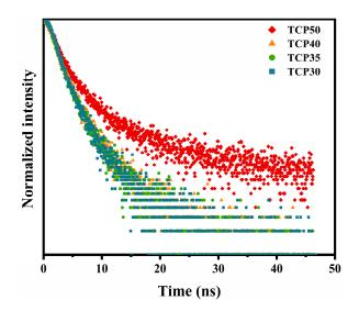
Figure 3. Fluorescence decay curve of TCPZ glasses at 530 nm.
