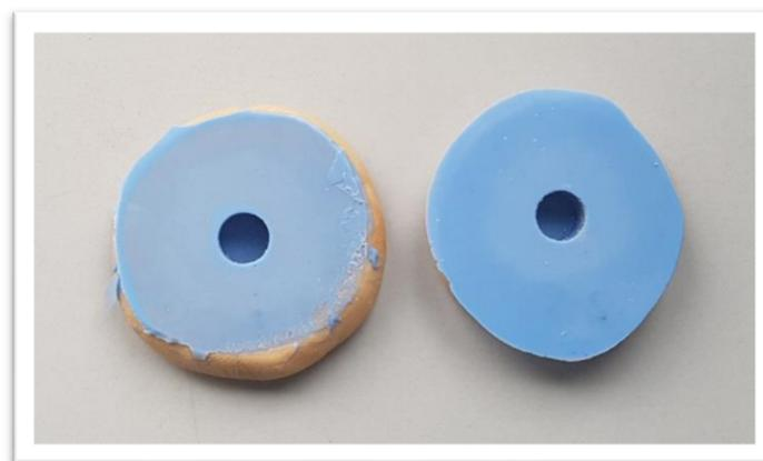
**Figure 2.** Molds (6 mm in diameter  $\times$  6 mm in height), corresponding to the size of metallic cylinders, were fabricated from dental silicone-based impression materials. The material was filled into each cylindrical hole with a slight excess. A glass slab was then placed on top of the filled molds and pressed down to remove the excess material.
