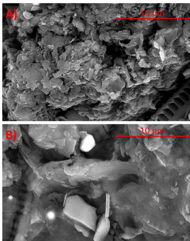
**Figure 5.** SEM images of “(A)” raw sludge and “(B)” sludge conditioned using the nIC-Conditioner catalyst composite.
