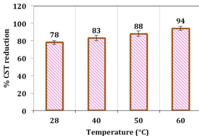
Figure 9. CST reduction efficiency linked to temperature effect using nIC-Conditioner/H<sub>2</sub>O<sub>2</sub>.
