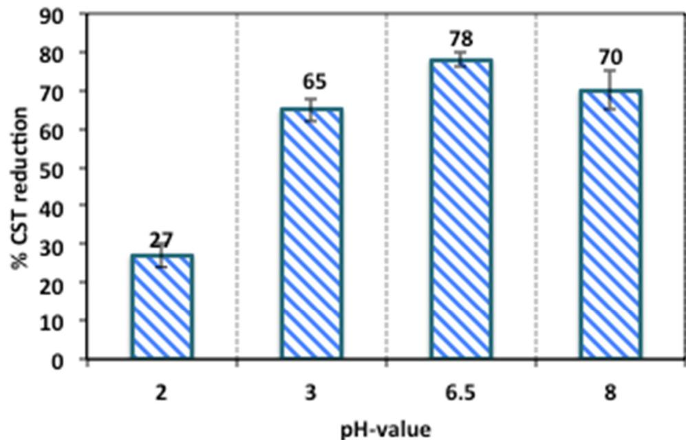
Figure 8. CST reduction efficiency linked to sludge pH using nIC-Conditioner/H<sub>2</sub>O<sub>2</sub>.
