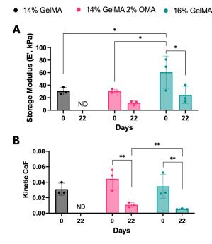
**Figure 11.** Mechanical characterization of 3D bioprinted groups. (**A**) Storage modulus determined by DMA (1 Hz). (**B**) Kinetic coefficient of friction determined by lap-shear testing. \*\* p value < 0.005 and \* p value < 0.05. ND = not determined. n = 3,  $\pm$  S.D.
