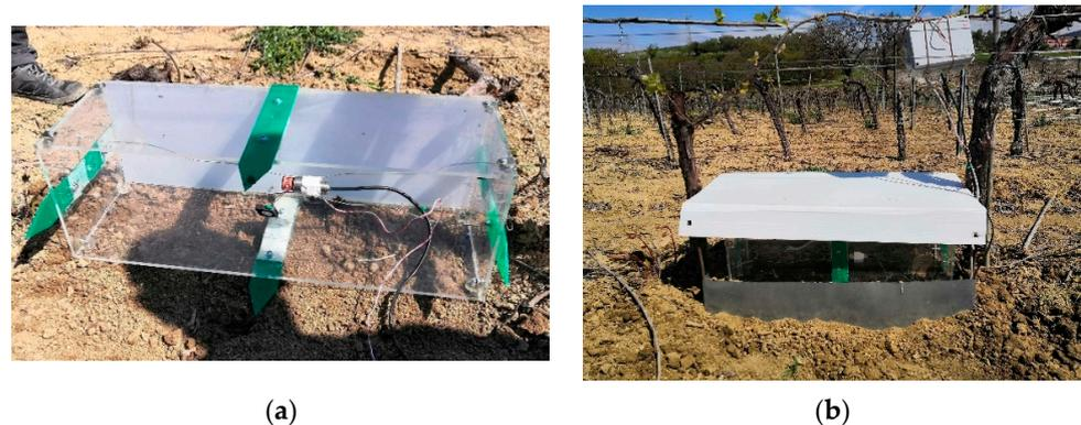
**Figure 2.** Structure of the soil respiration chamber prototypes (SRCps) (a) and the protective bulkheads (b).
